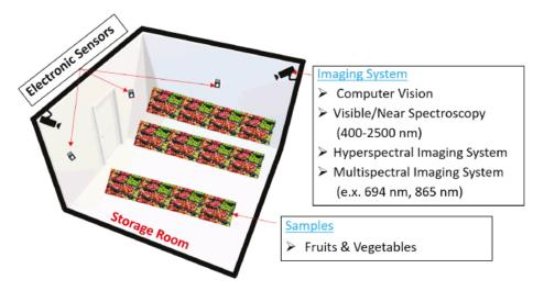
Figure 3. Schematics of multi-sensors coupled with imaging system for monitoring the quality of fruits and vegetables during cold storage.
