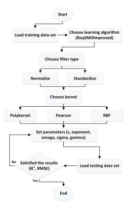
Figure 2. The workflow of support vector machine (SVM).
