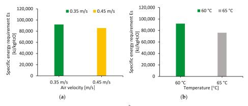
**Figure 16.** Specific energy requirements for 25 kg/m<sup>2</sup> bulk dried at (a) 0.35 m/s and 0.45 m/s at 60 °C (b) 60 °C and 65 °C at 0.35 m/s.
