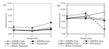
**Figure 7.** Changes in solid-non-fat of (**a**) cow and (**b**) goat milk during storage period of 22 days. Solid lines represent HPP-treated milk (450 MPa/7 min, 600 MPa/5 min, 600 MPa/7 min), dashed lines represent pasteurized milk, and dotted lines represent fresh milk before treatment.
