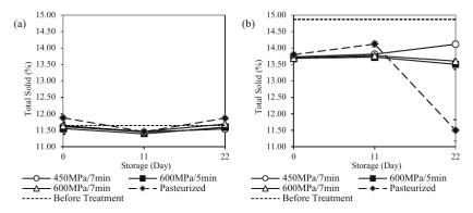
**Figure 6.** Changes in total solid of (**a**) cow and (**b**) goat milk during storage period of 22 days. Solid lines represent HPP-treated milk (450 MPa/7 min, 600 MPa/5 min, 600 MPa/7 min), dashed lines represent pasteurized milk, and dotted lines represent fresh milk before treatment.
