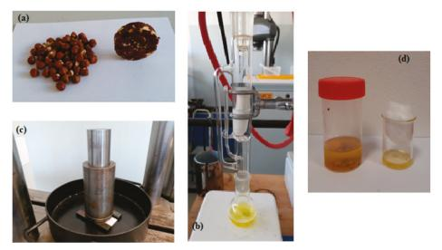
**Figure 1.** Set up of compression test and Soxhlet extraction: (a) hazelnut kernels and seed cake after compression; (b) Soxhlet extraction setup for kernel oil content determination; (c) a pan holding the pressing vessel with a plunger placed on two separated metal bars with a piece of white paper for oil point identification similar for the compression test; and (d) hazelnut kernel oil from the compression test and Soxhlet extraction (covered with cotton wool).
