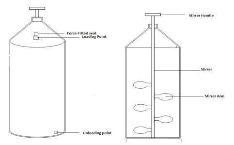
Figure 1. Schematic view of the locally developed aluminum storage silo.
