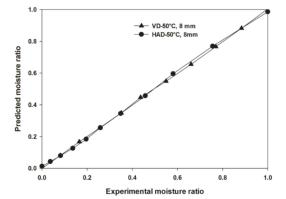
Figure 5. Predicted versus experimental moisture ratio data for logarithmic model at 50  $^{\circ}\mathrm{C}$  and 8 mm samples thickness for VD and HAD methods.
