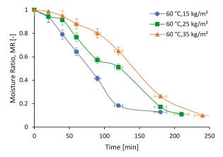
Figure 5. Moisture ratio (MR) vs. time (min) for hops with three different bulk weights dried at 60  $^{\circ}$ C and 0.35 m/s.
