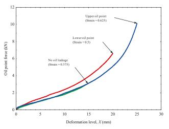
Figure 4. Oil point identification at deformation levels of bulk hazelnut kernels.
