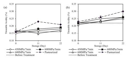
**Figure 2.** Changes in titratable acidity of (**a**) cow and (**b**) goat milk during storage period of 22 days. Solid lines represent HPP-treated milk (450 MPa/7 min, 600 MPa/5 min, 600 MPa/7 min), dashed lines represent pasteurized milk, and dotted lines represent fresh milk before treatment.
