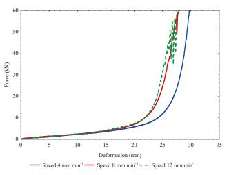
Figure 2. Force-deformation curves of bulk hazelnut kernels for different speeds.
