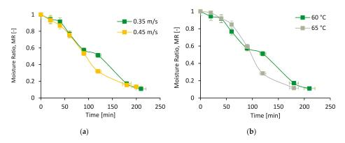
**Figure 6.** Moisture ratio (MR) vs. time (min) for hops dried at (a) 0.35 m/s and 0.45 m/s at 60  $^{\circ}$ C (b) 60  $^{\circ}$ C and 65  $^{\circ}$ C at 0.35 m/s.
