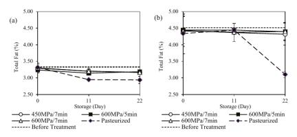
**Figure 5.** Changes in total fat of (**a**) cow and (**b**) goat milk during storage period of 22 days. Solid lines represent HPP-treated milk (450 MPa/7 min, 600 MPa/5 min, 600 MPa/7 min), dashed lines represent pasteurized milk, and dotted lines represent fresh milk before treatment.
