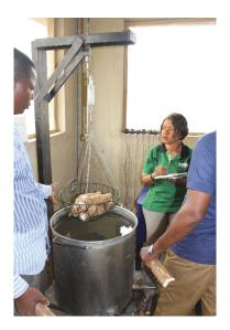
**Figure 2.** Reimann Balance (Specific Gravity) Method as constructed at the Federal University of Agriculture, Abeokuta, Nigeria.
