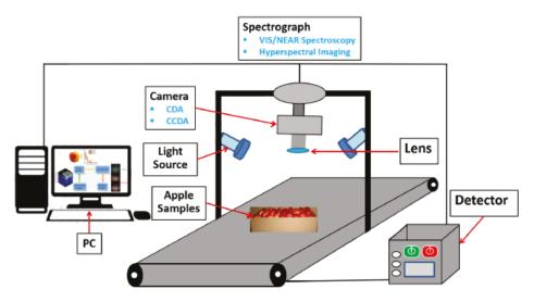
Figure 2. Typical set-up of an imaging system for monitoring the quality of fresh agricultural produce.
