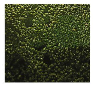
**Figure 7.** Air channel formation in a 15 kg/m<sup>2</sup> bulk of hops.
