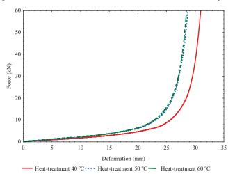
Figure 3. Force-deformation curves of bulk hazelnut kernels for heating temperatures.Table 4. Strain and oil point force of deformation levels of kernels at a speed of 4 mm/min.
