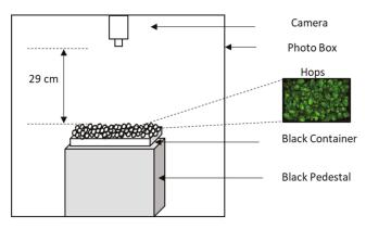
Figure 3. Schematic of RGB camera imaging system for hops.
