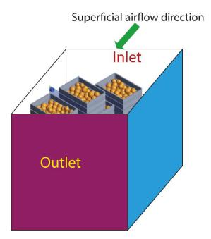
**Figure 4.** Simulation domain showing loaded fruits in stacked cartons in a virtual wind tunnel system with internal and external surrounding conditions [101].
