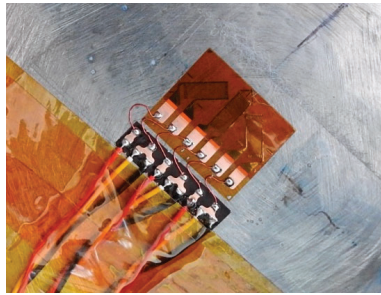
Figure 11. Foil strain gauge with adjacent solder tabs.
