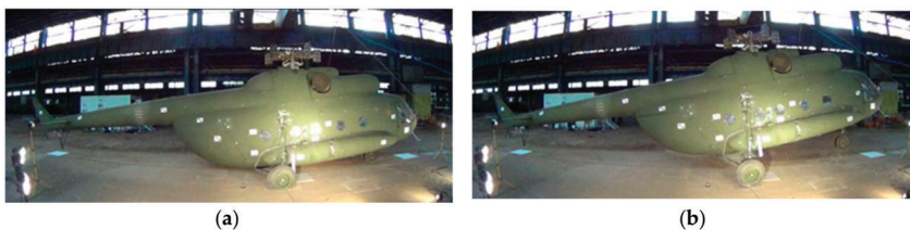
Figure 2. Experimental activity. Helicopter during: maximum strut compression (a) and front-wheel spring back (b).
