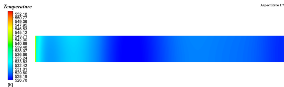
Figure 9. Temperature of chemical reaction zone (2.5 kW heat flux).
