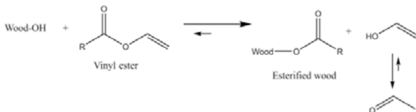
Figure 8: Acetylation of wood with vinyl acetate
