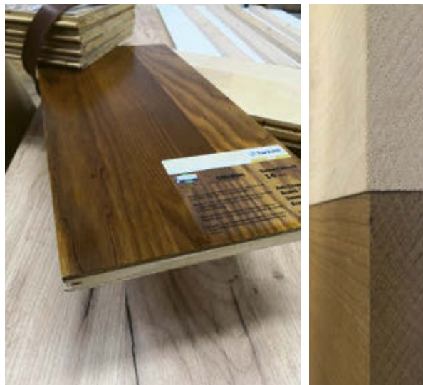
Figure 37: Thermal modified ash wood flooring (top layer), and maple wood, treated and untreated (right)
