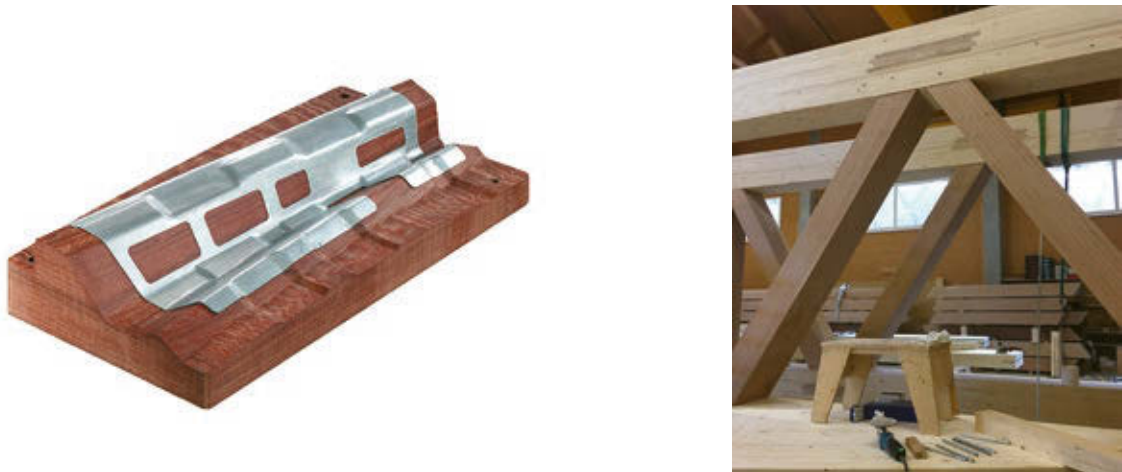
Figure 24: Densified resin-impregnated and laminated beech veneer from Deutsche Holzveredelung Schmeing GmbH & Co. KG (left), and BauBuche from Pollmeier Massivholz GmbH & Co. KG in a fram construction under construction at Neue Holzbau AG Lungern (right)
