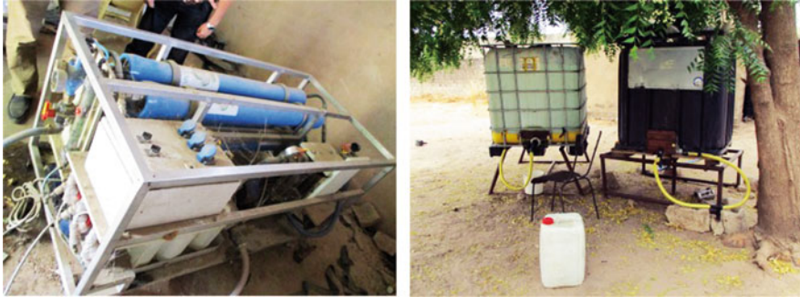
Fig. 4.6 Water purification device with a reverse osmosis membrane filter and a 20 L plastic container filled with filtered water for sale. (Photos by Ikemi)
