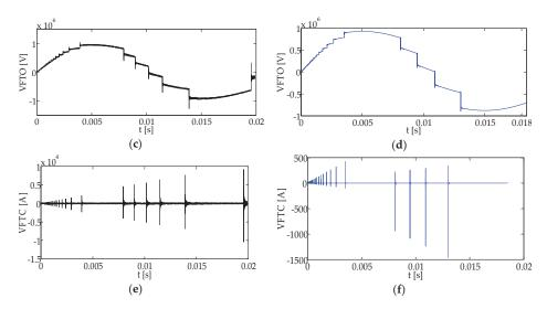
Figure 7. Very fast transient overvoltage (VFTO) and VFTC waveforms: VFTO at the source side (a) before installing the damping busbar and (b) after installing it; VFTO at the load side (c) before installing the damping busbar and (d) after installing it; VFTC (e) before installing the damping busbar and (f) after installing it.
