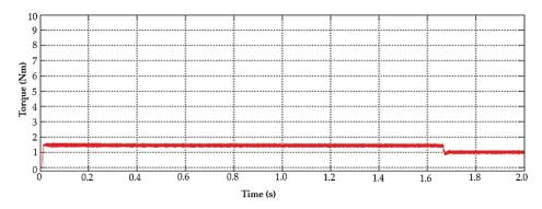
Figure 12. Output load torque characteristics of the BLDC motor after using the LUO converter.
