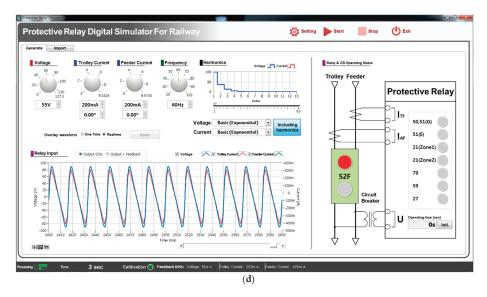
Figure 20. Simulation results for Case 5: (a) Input current; (b) Input voltage; (c) Protective relay signal; and (d) Digital simulator interface results.
