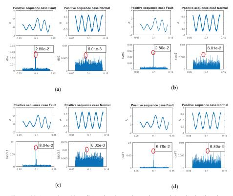
**Figure 9.** Maximum values of the coefficients from the wavelet transform at scale 2 used in classifying the faults in relay 2: (a) Daubechies (db2); (b) symlets (sym2); (c) biorthogonal (bior3.1); (d) Coiflets (coif1).
