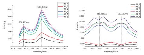
**Figure 3.** Emission intensity of Na in samples #1-1 through #1-6 measured at different wavelengths at an energy intensity of 3.8 J/cm<sup>2</sup>. Spectra show the resonance lines (588.995 nm, 589.592 nm) and nonresonant lines (568.263 nm, 568.859 nm).
