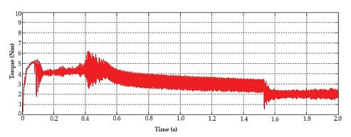
Figure 11. Output load torque characteristics of the BLDC motor before using the LUO converter.
