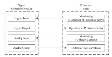
**Figure 3.** Signal generation and each function of the collecting part.
