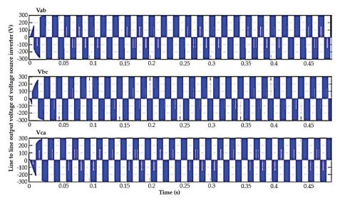
Figure 7. The output waveform of the voltage source inverter.
