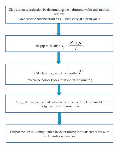
Figure 9. The flowchart of the procedure to calculate the litz coil design.
