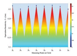
Figure 13. Equivalent resistivity  $\rho_r$  related to Figure 11. The large size of meshes  $M_1$  and  $M_2$  results in weak magnetic coupling and, therefore,  $\rho_r$  at  $P_4$  and  $P_6$  is higher than  $\rho_r$  at  $P_2$  and  $P_8$ .
