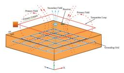
**Figure 4.** A typical transient electromagnetic method (TEM) system probing the underground grid. The primary magnetic field due to the transmitter coil interacts with the grid buried in the soil and induces eddy currents. Induced eddy currents produce a secondary magnetic field that travels upward to the Earth's surface and collected by the receiver coil placed in the center of the transmitter coil.
