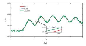
**Figure 3.** Comparison of G1 state filtering results under ensemble Kalman filter (EnKF) and AEnSRF: (a) Power angle dynamic estimation curve of G1; (b) electric angular velocity dynamic estimation curve of G1.
