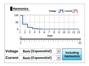
Figure 8. Internal waveform generation including harmonics.
