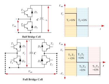
**Figure 6.** A schematic of the configuration of the MMC based on half-bridge and full-bridge sub-modules (SMs).
