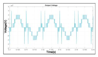
Figure 1. Voltage for a single AC side cascaded configuration including two H-bridges [26].
