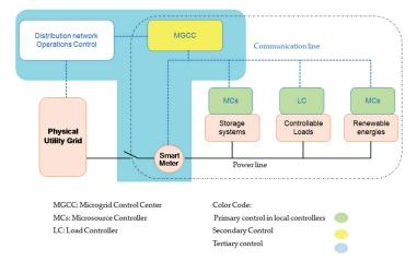
Figure 3. Modern basic structure of a microgrid.
