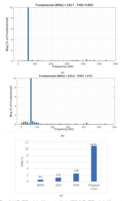
Figure~16.~(a)~ The~THD~ analysis~ of~ the~ current~ grid~ using~ HHO; (b)~ The~ THD~ analysis~ of~ the~ current~ grid~ using~ ASO; (c)~ Comparison~ between~ the~ THD~ analysis~ of~ the~ current~ grid~ with~ different~ methods.
