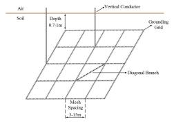
Figure 1. Grounding grid and its characteristics.
