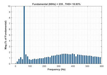
Figure 15. Total harmonic distortion (THD) analysis of the grid current in the original case.
