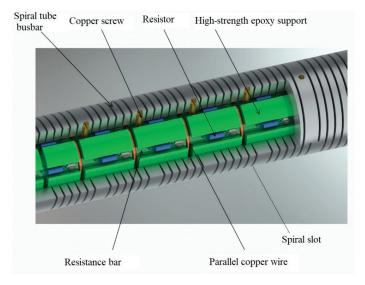
Figure 2. The structure of the damping busbar.
