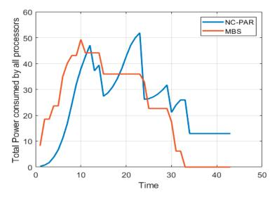
Figure 8. Total power consumed by all processors using MBS and NC-PAR.
