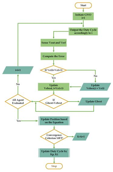
**Figure 3.** Flow chart of the Grey Wolf Optimizer (GWO)-based Maximum Power Point Tracking (MPPT) algorithm.
