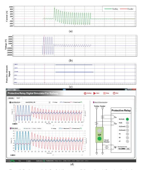
$\label{eq:Figure 17.} \textbf{Figure 17. Simulation results for Case 3: (a) Input current; (b) Input voltage; (c) Protective relay signal; and (d) Digital simulator interface results.}$
