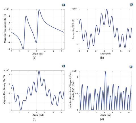
**Figure 3.** Influence of the surrounding electromagnetic environment (EME) on the derivative method. (a) Surface magnetic flux density  $\vec{B_z}$  pertaining to the grounding grid in [26]. (b) Surrounding EME. (c) Mixed signal  $\vec{M_z}$  of magnetic flux density  $\vec{B_z}$  and the surrounding EME. (d) Derivative of mixed signal  $\vec{M_z}$ . This signal contains fake peaks due to the presence of EME, which causes the identification of true peaks to be impossible.
