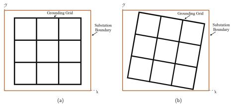
Figure 2. Grounding grid orientation with respect to the substation boundary. (a) Grounding grid oriented parallel along the substation boundary. (b) Grounding grid with non-parallel orientation along the substation boundary.
