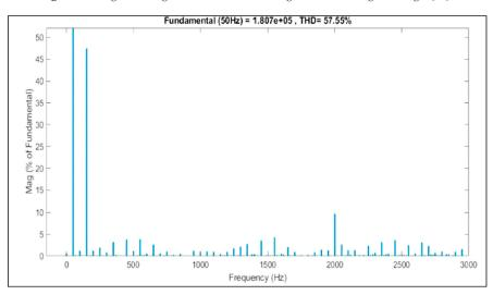
Figure 4. A representation of the harmonic component in the output voltage of the AC side cascaded configuration using 4H-bridges [26].
