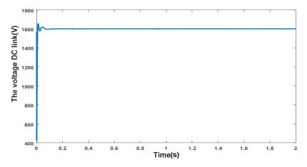
Figure 24. The voltage DC link of the MMC with an imbalanced load.
