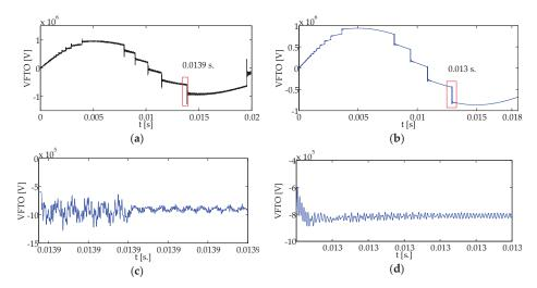
**Figure 10.** VFTO waveform at the load side: (a) before installing the damping busbar, (b) after installing the improved design of the damping busbar; VFTO at the load side for one breakdown at 0.013 s: (c) before installing the damping busbar, (d) after installing the improved design of the damping busbar.
