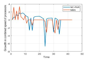
Figure 7. Growth of combined speed of all processors using MBS and NC-PAR.
