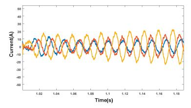
Figure 21. The current at the grid side with an imbalanced load.
