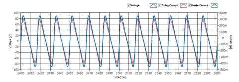
Figure 19. Current waveform with harmonics.
