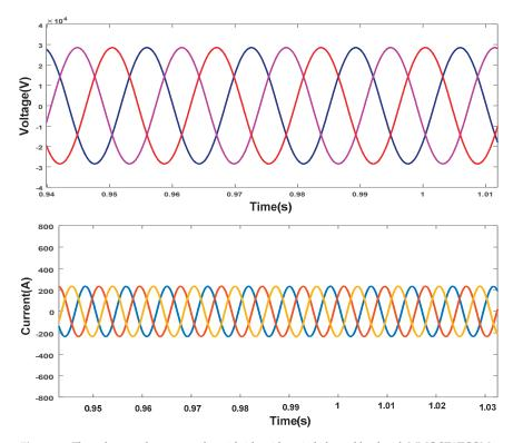
Figure 23. The voltage and current at the grid side with an imbalanced load with MMC STATCOM.
