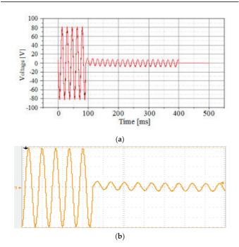
**Figure 10.** COMTRADE Output waveform test: (a) COMTRADE input waveform; (b) Simulator output waveform (voltage: 20 V/Div, time: 25 ms/Div).
