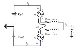
Figure 7. The one phase equivalent circuit.
