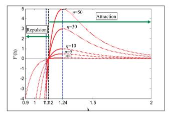
**Figure 12.** The behavior of the interaction force function with the scaled distance (*h*) under different depth values [34].
