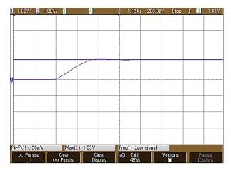
Figure 21. Speed waveform of the BLDC motor.
