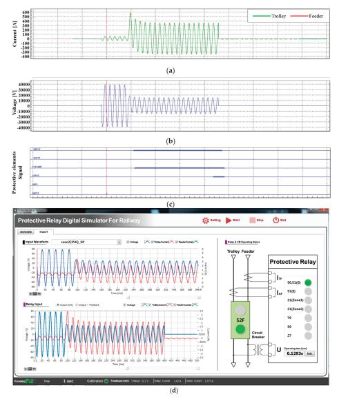
Figure 16. Simulation results for Case 2: (a) Input current; (b) Input voltage; (c) Protective relay signal; and (d) Digital simulator interface results.
