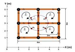
**Figure 5.** Simulation model featuring the square grounding grid of dimensions  $4 \text{ m} \times 4 \text{ m}$  and mesh spacing 2 m. Conductors are labeled  $C_1$  to  $C_{12}$  and nodes 1 to 9.  $I_1$  to  $I_4$  are the induced eddy currents whose direction of flow is indicated by arrows. The TEM system is moved 0.05 m above the surface along circle of radius 1 m from point  $P_1$  to  $P_8$ .
