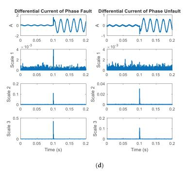
**Figure 4.** Differential current signals from the wavelet transform in the case of internal faults at phases in each mother wavelet: (a) Daubechies (db2); (b) symlets (sym2); (c) biorthogonal (bior3.1); (d) Coiflets (coif1).
