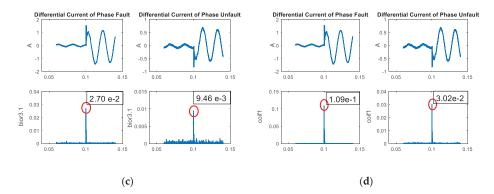
**Figure 8.** Maximum values of the coefficients from the wavelet transform at scale 2 used in classifying the faults in relay 1: (a) Daubechies (db2); (b) symlets (sym2); (c) biorthogonal (bior3.1); (d) Coiflets (coif1).
