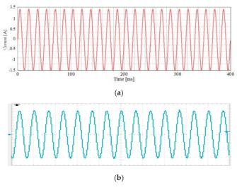
**Figure 11.** Customized waveform output test: (a) Simulator input waveform; (b) Simulator output waveform (voltage: 200 mV/div, time: 25 ms/div).
