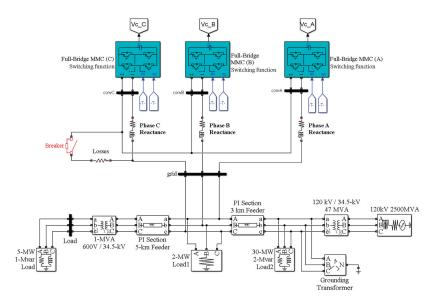
Figure 9. A model of the power system under study.
