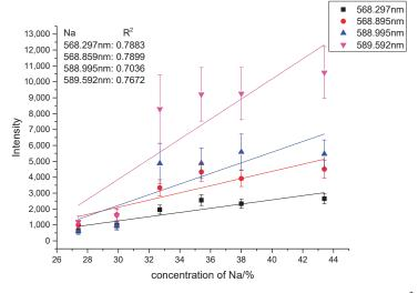
Figure 5. LIBS signal intensity of Na vs. Na concentration at a laser fluence of 3.8 J/cm<sup>2</sup>.
