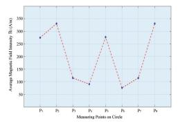
**Figure 12.** Average magnetic field intensity  $\overline{H_z}$  along  $P_1$  to  $P_8$  related to Figure 11. The large size of meshes  $M_1$  and  $M_2$  results in weak magnetic coupling, and therefore,  $\overline{H_z}$  at  $P_4$  and  $P_6$  is less than  $\overline{H_z}$  at  $P_2$  and  $P_8$ .
