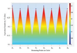
**Figure 6.** Equivalent resistivity  $\rho_r$  along the circle from  $P_1$  to  $P_8$ . High  $\rho_r$  at  $P_1$ ,  $P_3$ ,  $P_5$ , and  $P_7$  corresponds to the presence of conductors  $C_4$ ,  $C_{10}$ ,  $C_3$ , and  $C_9$ .  $C_4$  at 0 rad,  $C_{10}$  at 1.57 rad,  $C_3$  at 3.14 rad, and  $C_9$  at 4.71 rad along the circle showed the parallel orientation of the grid in the plane.
