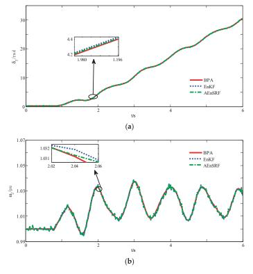
**Figure 5.** Comparisons of G2 state filtering results between EnKF and AEnSRF in the presence of measurement noise deviation: (a) Power angle dynamic estimation curve of G2; (b) electric angular velocity dynamic estimation curve of G2.
