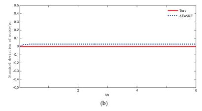
**Figure 8.** Tracking curve of AEnSRF for generator measurement noise with deviation of measurement noise: (a) Power angle measurement noise tracking curve of generator; (b) angular velocity measurement noise tracking curve of generator.
