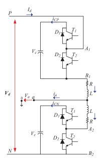
Figure 8. The one phase equivalent circuit of the MMC static synchronous compensator (STATCOM).
