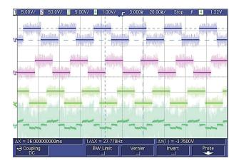
Figure 18. Hall sensor signals and stator current waveform of the BLDC motor.
