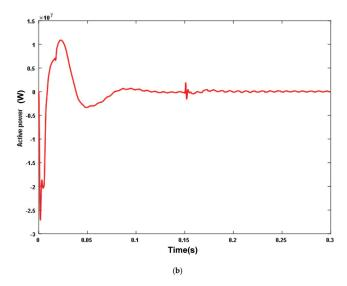
**Figure 19.** The reactive and active power with connection to the MMC STATCOM. (a) Reactive power; (b) Active power.
