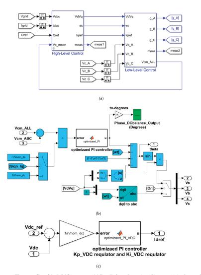
**Figure 10.** The controller of the MMC converter: (a) Simulink configuration; (b) An optimized controller for phase balancing based on the Harris hawk's optimization (HHO) or Atom search optimization (ASO) optimization techniques; (c) An optimized controller of DC voltage based on the HHO or ASO optimization techniques.
