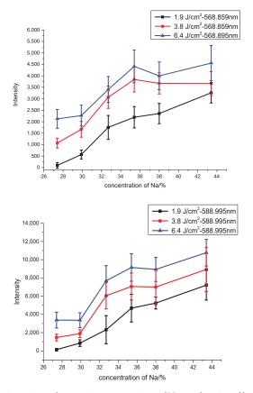
Figure 4. Emission intensity under varying concentrations of Na as a function of laser energy. Signals obtained from the Na I 588.995 nm, Na I 568.859 nm are shown.
