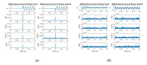
**Figure 6.** Differential current signals from wavelet transform in scale 2 obtained from relay 1: (a) internal fault; (b) external fault.
