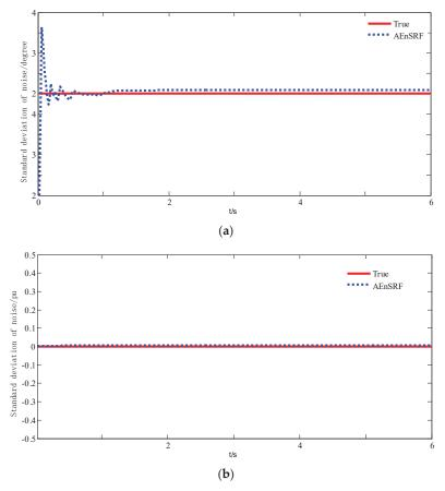
**Figure 6.** Tracking curve of G2 measurement noise by AEnSRF in the case of measurement noise deviation: (a) Power angle measurement noise tracking curve of G2; (b) angular velocity measurement noise tracking curve of G2.
