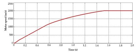
Figure 10. Steady-state response of the BLDC motor speed.
