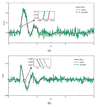
**Figure 7.** Contrast chart of EnKF and AEnSRF for generator state filtering with deviation of measurement noise: (a) Power angle dynamic estimation curve of generator; (b) dynamic angular velocity estimation curve of generator.
