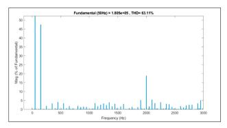
**Figure 2.** A representation of the harmonic component in the output voltage of the AC side cascaded configuration using two H-bridges [26].
