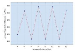
**Figure 7.** Average magnetic field intensity  $\overline{H_z}$  along the circle from  $P_1$  to  $P_8$ .  $\overline{H_z}$  is low at  $P_1$ ,  $P_3$ ,  $P_5$ , and  $P_7$ , confirming the presence of  $C_4$ ,  $C_{10}$ ,  $C_3$  and  $C_9$ , and the parallel orientation of the grid in the plane of the Earth.
