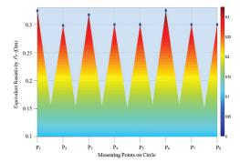
**Figure 9.** Equivalent resistivity  $\rho_r$  of Figure 8. High  $\rho_r$  at  $P_6$  validates the presence of diagonal conductor  $C_{13}$ . Unequal magnetic coupling due to an unequal mesh size results in low  $\rho_r$  at  $P_5$  and  $P_7$ .
