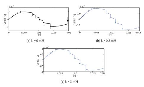
Figure 8. Influence of the inductance value on VFTO suppression at the load side of a 1000 kV GIS: at inductance values (a) L = 0 mH, (b) L = 0.3 mH, (c) L = 3 mH.
