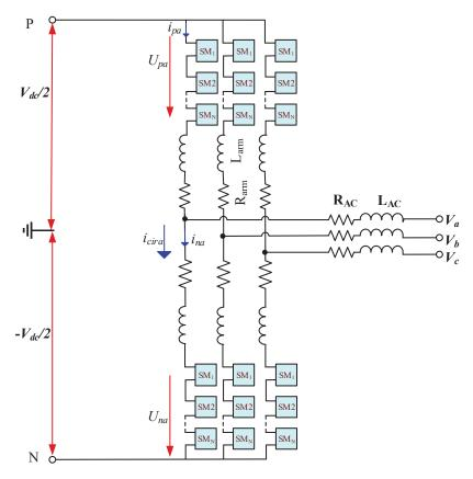
Figure 5. The circuit configuration of the MMC.
