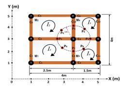
**Figure 11.** Grounding grid with an unequal mesh configuration. The dimensions of meshes  $M_1$  and  $M_2$  are 2.5 m  $\times$  2 m and  $M_3$  and  $M_4$  are 1.5 m  $\times$  2 m.
