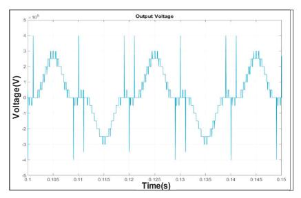
Figure 3. Voltage for a single AC side cascaded configuration including 4H-bridges [26].
