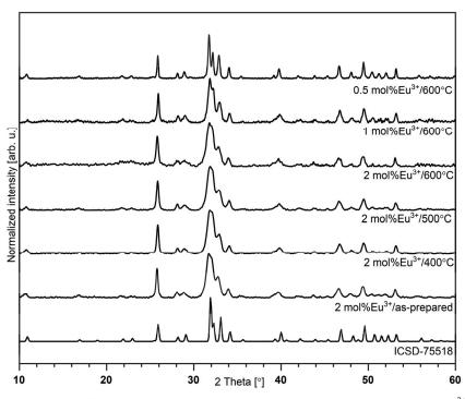
Figure 1. X-ray diffraction pattern of silicate-substituted hydroxyapatite co-doped with 2 mol%  $Sr^{2+}$  and x mol%  $Eu^{3+}$  ions.
