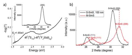
**Figure 2.** Basic properties of the deposited SmS and EuS thin films. (**a**) Optical (on glass) and structural (inset, on Si wafer) fingerprint of a 25 nm as-deposited EuS. (**b**) XRD patterns showing the structural behavior in the as-deposited (black line) S-SmS, as well as in the metallic state (red line), after rubbing. The lattice planes are indicated. In both thin film depositions, the substrate temperature was 250 °C.
