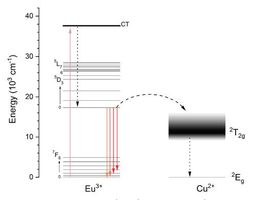
Figure 10. Simplified energy level scheme of Eu<sup>3+</sup> and Cu<sup>2+</sup> explaining quenching of Eu<sup>3+</sup> ion emission.
