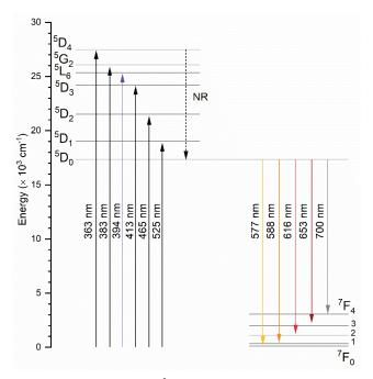
Figure 6. The simplified energy level scheme for Eu<sup>3+</sup> ion in silicate-substituted strontium-doped hydroxyapatite.
