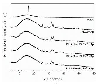
**Figure 3.** X-ray diffraction patterns of PLLA/x mol%  $Eu^{3+}$ :HAp composites (where x = 0-5) obtained with the extrusion method.
