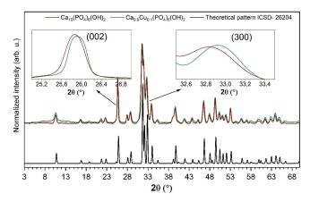
**Figure 1.** X-ray diffraction patterns of pure nanohydroxyapatite (nHAp) and nHAp doped with 1 mol%  $Cu^{2+}$  after heat treatment at 400 °C with the indication of (002) and (300) planes shift induced by doping with  $Cu^{2+}$  ions.
