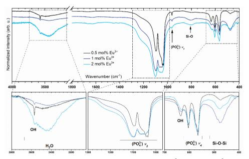
Figure 2. FT-IR spectra of the silicate-substituted hydroxyapatite co-doped with  $Sr^{2+}$  (2.0 mol%) and  $Eu^{3+}$  (0.5, 1.0 and 2.0 mol%) ions. 175
