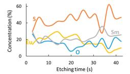
Figure 9. XPS depth profiling for the 6/12/6 nm SmS/EuS/SmS tri-layer system deposited at 400 °C.
