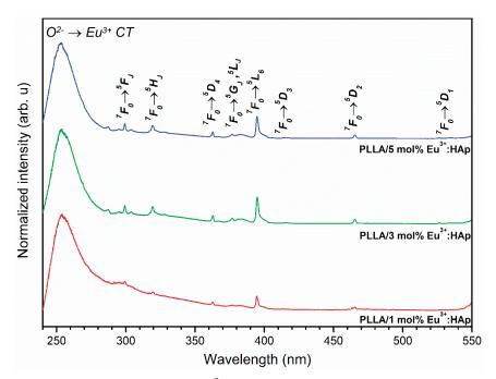
**Figure 6.** Excitation spectra of x mol%  $Eu^{3+}$ :HAp nanoparticles (where x = 1–5) incorporated into PLLA composites.
