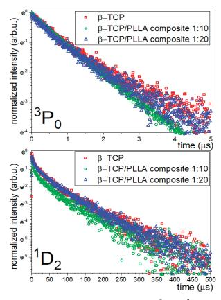
**Figure 6.** Luminescence kinetics curves of β-TCP co-doped with Ce<sup>3+</sup> and Pr<sup>3+</sup> ions PLLA with β-TCP composite with phosphate: polymer 1:10 ratio and PLLA with β-TCP composite with phosphate: polymer 1:20 ratio, recorded at 650 nm ( ${}^{3}P_{0}$ ) and recorded at 605 nm ( ${}^{1}D_{2}$ ).
