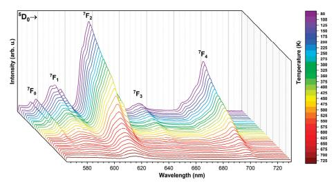
Figure 7. Temperature-dependent emission spectra of the Ca<sub>9.6</sub>Sr<sub>0.2</sub>Eu<sub>0.2</sub>(PO<sub>4</sub>)<sub>2</sub>(SiO<sub>4</sub>)<sub>4</sub>(OH)<sub>2</sub>, sintered at 600 °C.
