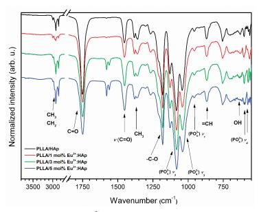
Figure 4. IR spectra of PLLA/x mol%  $Eu^{3+}$ :HAp composites (where x = 0–5) obtained via extrusion in situ.
