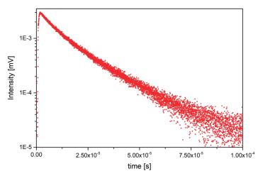
Figure 5. Decay time measured for 15 mol% Yb<sup>3+</sup>, 1 mol% Er<sup>3+</sup>:β-KYP<sub>2</sub>O<sub>7</sub> annealed at 650 °C for 12 h.
