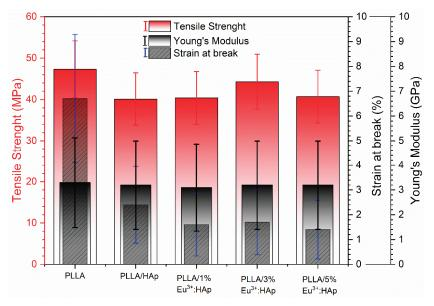
**Figure 9.** Tensile properties for PLLA/HAp composites: tensile strength (red left axis), strain at break (right axis) and Young's modulus (right axis).
