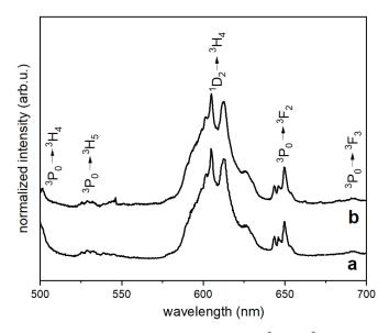
**Figure 5.** Emission spectra of PLLA with  $\beta$ -TCP co-doped with Ce<sup>3+</sup> and Pr<sup>3+</sup> ions (**a**) and PLLA with  $\beta$ -TCP composite with phosphate:polymer 1:20 ratio (**b**). Spectra were recorded after excitation with 445 nm.
