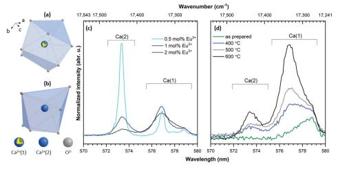
into account all results, one can note that in the silicate-substituted strontium-doped hydroxyapatite matrix, the Ca(1) site is more occupied by  $Eu^{3+}$  ions.
