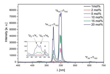
**Figure 4.** Representative emission spectra of KYP<sub>2</sub>O<sub>7</sub> doped with *x* mol% Yb<sup>3+</sup> ions and co-doped with 1 mol%  $\text{Er}^{3+}$  under the excitation wavelength  $\lambda = 980$  nm, *P* = 1.56 W, heat-treated at 650 °C for 12 h.
