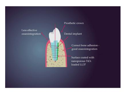
Figure 5. Ascheme showing difference in osseointegration between implant surface with and without coating.
