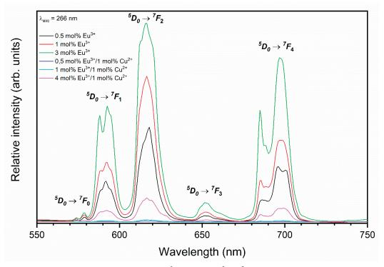
Figure 7. The emission spectra of the Eu<sup>3+</sup>-doped and Eu<sup>3+</sup>/Cu<sup>2+</sup> co-doped Ca<sub>10</sub>(PO<sub>4</sub>)<sub>6</sub>(OH)<sub>2</sub>.
