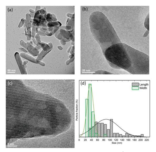
Figure 3. Representative TEM images (a-c) and particle size distribution (d) of the 1 mol% Eu<sup>3+</sup>:Ca<sub>10</sub>(PO<sub>4</sub>)<sub>6</sub>(OH)<sub>2</sub>.
