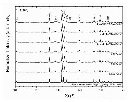
Figure 1. X-ray powder diffraction patterns of the  $Eu^{3+}$ -doped and  $Eu^{3+}/Cu^{2+}$  co-doped  $Ca_{10}(PO_4)_6(OH)_2$ .
