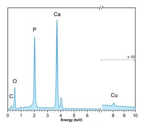
Figure 5. EDS spectrum of nHAp doped with 1 mol% Cu<sup>2+</sup> after heat treatment at 400 °C.
