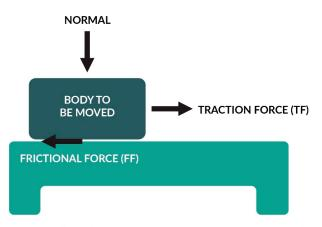
**Figure 3.** Different forces acting over a body under traction on top of a surface. Body to be moved, traction force (TF), friction force (FF), contact surface (CS).
