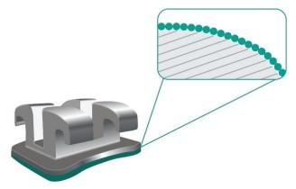
Figure 4. Orthodontic bracket covered by a nano-sized film.
