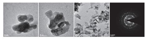
Figure 1. Representative TEM images and a SAED image of the 3 mol% Eu<sup>3+</sup>:Ca<sub>10</sub>(PO<sub>4</sub>)<sub>6</sub>(OH)<sub>2</sub>.
