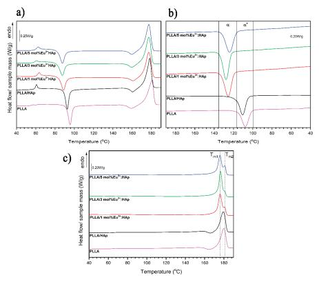
Figure 5. The first heating (a), cooling (b) and second heating (c) DSC curves of PLLA and PLLA/x mol%  $Eu^{3+}$ :HAp composites (where x = 0–5).
