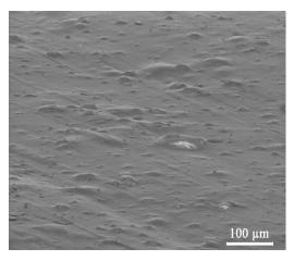
Figure 2. SEM image of composite surface for PLLA/HAp.
