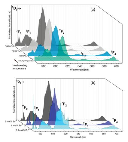
Figure 4. Emission spectra of  $Ca_{9.6}Sr_{0.2}Eu_{0.2}(PO_4)_2(SiO_4)_4(OH)_2$  as a function of sintering temperature (a) and  $Ca_{9.8-x}Sr_{0.2}Eu_x(PO_4)_2(SiO_4)_4(OH)_2$ , where x = 0.5, 1.0, 2.0 mol%, sintered at 600 °C (b).
