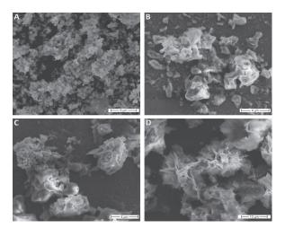
Figure 4. SEM images of (A)  $\beta$ -TCPco-doped with Ce<sup>3+</sup> and Pr<sup>3+</sup> ions, (B) PLLA, (C) PLLA with  $\beta$ -TCP composite with phosphate:polymer 1:10 ratio, and (D) PLLA with  $\beta$ -TCP composite with phosphate:polymer 1:20 ratio.
