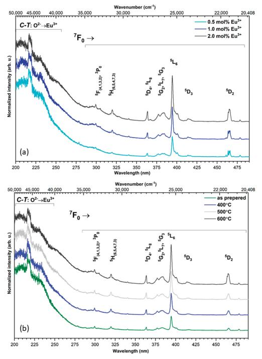
**Figure 3.** Excitation emission spectra of  $Ca_{9.8-x}Sr_{0.2}Eu_x(PO_4)_2(SiO_4)_4(OH)_2$ , where x = 0.5, 1.0, 2.0 mol%, sintered at 600 °C (a) as well as  $Ca_{9.6}Sr_{0.2}Eu_{0.2}(PO_4)_2(SiO_4)_4(OH)_2$  as a function of sintering temperature (b).
