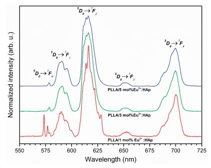
**Figure 7.** Emission spectra of PLLA/x mol%  $Eu^{3+}$ :HAp composites (where x = 0–5) incorporated into poly(L-lactide) composites obtained by using the extrusion method.
