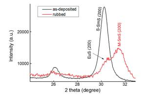
Figure 3. XRD patterns of an as-deposited SmS/EuS/SmS (35/30/35 nm) tri-layer deposited at 250 °C (black curve), and after rubbing (red curve).
