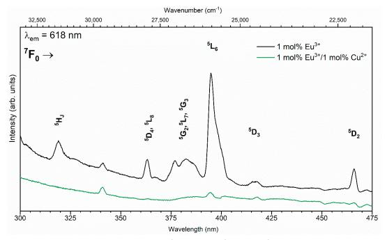
Figure 6. The excitation spectra of the 1 mol% Eu<sup>3+</sup> and 1 mol% Eu<sup>3+</sup>/1 mol% Cu<sup>2+</sup>-co-doped Ca<sub>10</sub>(PO<sub>4</sub>)<sub>6</sub>(OH)<sub>2</sub>.
