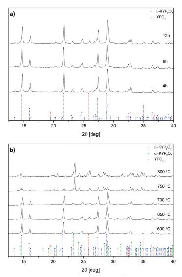
**Figure 2.** Representative XRD patterns of 1 mol%  $Er^{3+}$ , 1 mol%  $Yb^{3+}$ :KYP<sub>2</sub>O<sub>7</sub> annealed at 600 °C for 4, 8 and 12 h (**a**) as well as annealed at 600–800 °C for 4 h (**b**).
