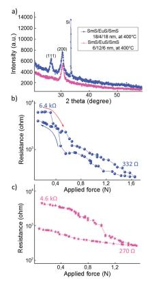
**Figure 8.** (a) XRD patterns of the thinner tri-layer systems (18/4/18 nm in blue dots and 6/12/6 nm in purple stars). Piezoresistance behavior for 18/4/18 nm tri-layer (b) and 6/12/6 nm tri-layer (c) deposited in between Ir electrodes. For clarity, in (b) red arrow represents the loading process, while the navy arrow shows the unloading process.
