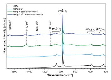
Figure 4. The micro-Raman spectra of nHAp and nHAp doped with 1 mol% Cu<sup>2+</sup> as well as both materials loaded with ozonated olive oil.
