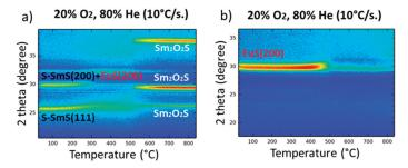
**Figure 4.** (a) In situ XRD patterns for increasing temperature of an as-deposited 35/30/35 nm SmS/EuS/SmS tri-layer in an ambient-like atmosphere of 20% O<sub>2</sub> and 80% He. (b) Same as in (a) for an as-deposited 25 nm EuS thin film on Si. Both thin films were deposited at 250 °C.
