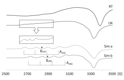
Figure 11. Experimental and simulated electron paramagnetic resonance (EPR) spectra of the 1 mol%  $Eu^{3+}/1$  mol%  $Cu^{2+}:Ca_{10}(PO_4)_6(OH)_2$ .
