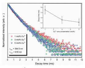
**Figure 8.** Emission kinetics of the  $Eu^{3+}$ : $Ca_{10}(PO_4)_6(OH)_2$  nanoparticles embedded into poly(L-lactide) composites obtained by using the extrusion method. Insert: The decay time as a function of  $Eu^{3+}$  ions concentration.
