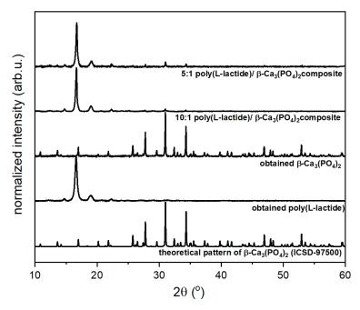
**Figure 1.** X-ray diffraction patters of poly(L-lactide) (PLLA),  $\beta$ -Ca<sub>3</sub>(PO<sub>4</sub>)<sub>2</sub> ( $\beta$ -TCP) co-doped with Ce<sup>3+</sup> and Pr<sup>3+</sup> ions and PLLA with  $\beta$ -Ca<sub>3</sub>(PO<sub>4</sub>)<sub>2</sub> composite compared to theoretical pattern of  $\beta$ -Ca<sub>3</sub>(PO<sub>4</sub>)<sub>2</sub> (ICSD-97500).
