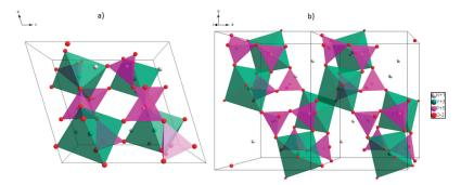
**Figure 1.** Projection of the  $\beta$ -KYP<sub>2</sub>O<sub>7</sub> unit cell (a) and super cell (b) indicating the Y<sup>3+</sup> and P<sup>5+</sup> coordination polyhedra.
