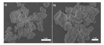
**Figure 3.** Representative SEM images of the 1 mol%  $Er^{3+}$ , 1 mol%  $Yb^{3+}$ : $KYP_2O_7$ , annealed at 600 °C for 12 h with different magnifications (**a**) with 3 um scale bar and (**b**) with 1 um scale bar.
