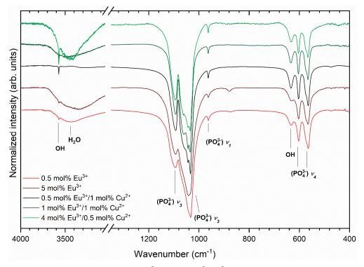
Figure 4. Infrared spectra of the Eu<sup>3+</sup>-doped and Eu<sup>3+</sup>/Cu<sup>2+</sup> co-doped Ca<sub>10</sub>(PO<sub>4</sub>)<sub>6</sub>(OH)<sub>2</sub>.
