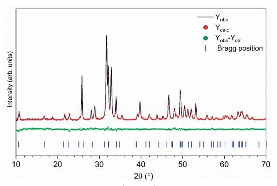
**Figure 2.** Representative results for the 0.5 mol%  $Eu^{3+}/1$  mol%  $Cu^{2+}$ : $Ca_{10}(PO_4)_6(OH)_2$ :, Rietveld analysis (red—fitted diffraction, green—differential pattern, and blue column—reference phase peak position).
