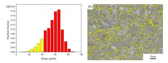
**Figure 8.** Fusion zone in the heat-treated joint (P = 2500 W, t = 5 ms): (**a**) Image quality in percentage showing highlighted low image quality and (**b**) Image quality map showing highlighted phases corresponding to martensite.
