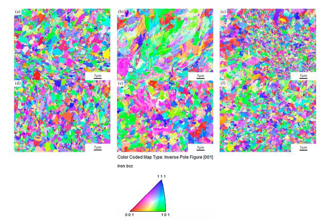
**Figure 6.** Inverse pole figure (IPF) maps of different regions: (a) base material, (b) fusion zone, (c) HAZ, (d) heat-treated base material, (e) heat-treated fusion zone and (f) heat-treated HAZ.
