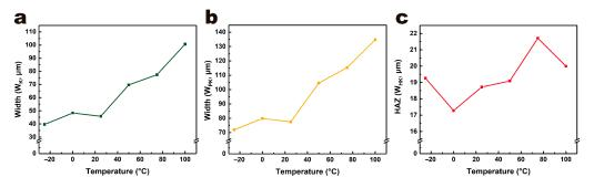
**Figure 11.** Kerf width (**a**), processing area width (**b**) and HAZ (**c**) of PET films at different ambient temperatures in line laser processing experiment.
