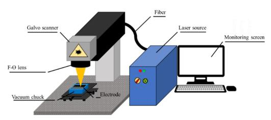
Figure 1. Set up of Ytterbium nanosecond Pulsed Fiber Laser used for laser structuring.
