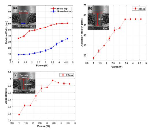
Figure 3. (a) Ablation width, (b) ablation depth, and (c) aspect ratio.
