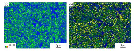
**Figure 9.** (a) Kernel average misorientation (KAM) map of the fusion zone in the heat-treated joint (P = 2500 W, t = 5 ms) and (b) Kernel average misorientation (KAM) map combined with image quality (IQ) map shown in Figure 8b.
