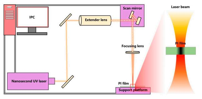
Figure 1. Experimental setup of PI film cutting process.
