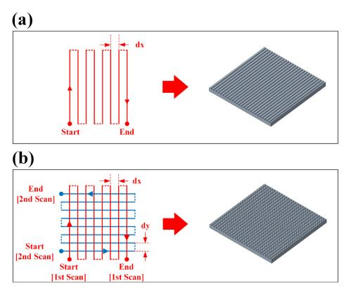
**Figure 1.** Pattern designs used for laser surface texturing of BMG: (**a**) unidirectional; (**b**) cross-hatch. **Table 1.** Processing parameters for the laser-based surface texturing experiments.
