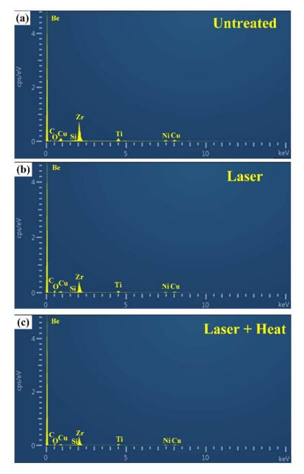
**Figure 7.** EDAX spectra for (**a**) untreated BMG surface; (**b**) laser textured BMG surface; (**c**) laser textured BMG surface followed by heat treatment.
