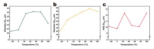
**Figure 9.** Hole diameter (**a**), processing area diameter (**b**) and HAZ (**c**) of PET films at different ambient temperature in the single spot laser processing experiment.
