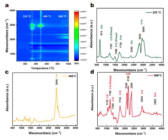
**Figure 5.** Infrared spectral intensity maps of evolved gaseous products during pyrolysis of PET film (**a**), and infrared spectrogram at typical temperatures: (**b**)  $335 \degree$ C, (**c**)  $489 \degree$ C and (**d**)  $996 \degree$ C.
