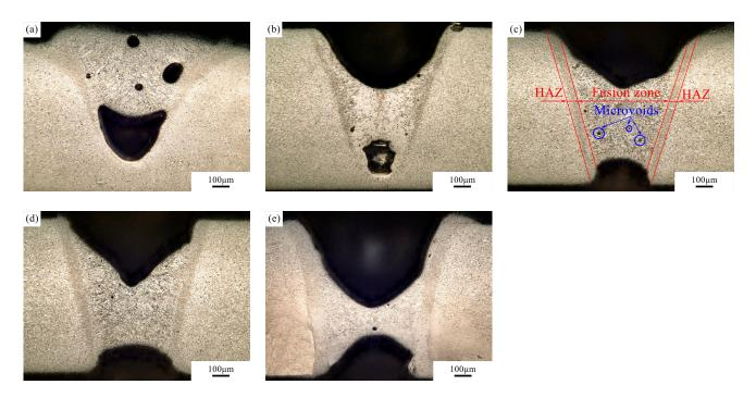
**Figure 3.** Optical micrographs of spots on the plate, with a power of 2500 W and a pulse duration of (**a**) 2 ms, (**b**) 2.5 ms, (**c**) 3 ms, (**d**) 3.5 ms and (**e**) 4 ms.
