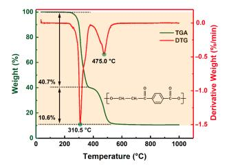
Figure 2. TGA-DTG curves of the PET film.
