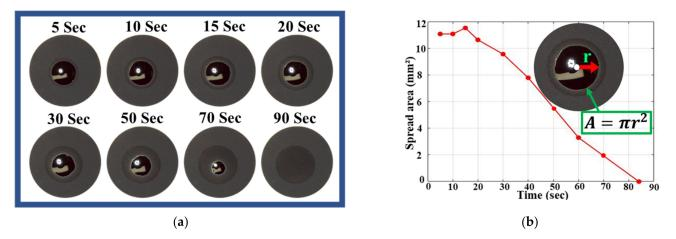
Figure 5. (a) Images of an unstructured electrode at different points in time. (b) Electrolyte spread over the unstructured electrode with time.
