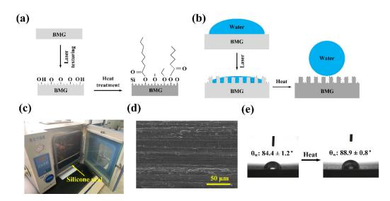
**Figure 12.** Schematic for the mechanism of wettability transition for the laser textured BMG surface after laser texturing and heat treatment: (**a**) alteration of surface chemistry; (**b**) alteration of surface wettability; (**c**) demonstration of the silicone seal on the furnace used in this work; (**d**) SEM micrograph of the untreated BMG surface; (**e**) contact angle measurement results for the untreated BMG surface before and after heat treatment.
