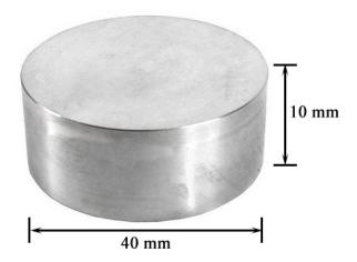
Figure 1. Powder metallurgy-produced ODS Eurofer.
