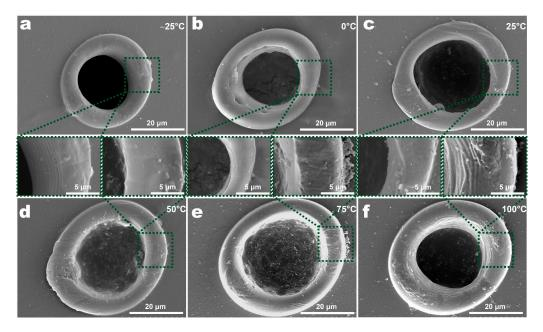
**Figure 8.** SEM images of holes of PET films at different ambient temperatures in the single-spot laser processing experiment: (**a**)  $-25 \degree$ C, (**b**)  $0 \degree$ C, (**c**)  $25 \degree$ C, (**d**)  $50 \degree$ C, (**e**)  $75 \degree$ C, (**f**)  $100 \degree$ C.
