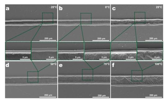
**Figure 10.** SEM images of kerfs of PET films at different ambient temperatures in line laser processing experiment: (a)  $-25 \degree$ C, (b)  $0 \degree$ C, (c)  $25 \degree$ C, (d)  $50 \degree$ C, (e)  $75 \degree$ C, (f)  $100 \degree$ C.
