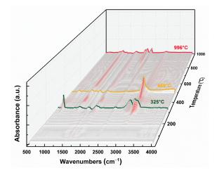
Figure 4. Infrared spectrogram of evolved gaseous products during pyrolysis of PET film.
