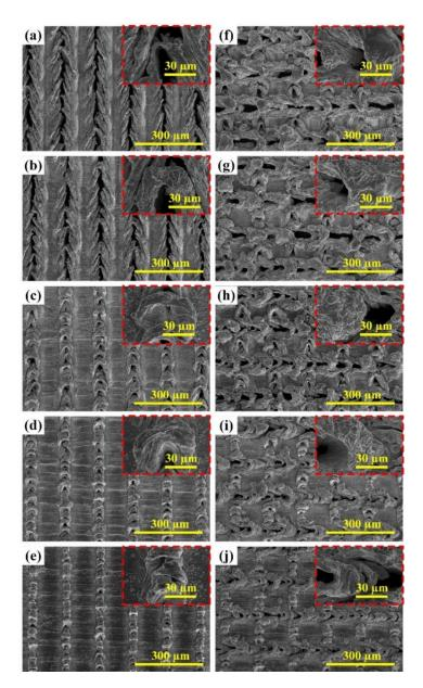
**Figure 4.** SEM micrographs of the laser textured BMG surfaces using different powers: (**a**–**e**) unidirectional surface patterns with the laser powers of 15.0 W, 13.5 W, 12.0 W, 10.5 W, and 9.0 W; (**f**–**j**) cross-hatch surface patterns with the laser powers of 15.0 W, 13.5 W, 12.0 W, 10.5 W, and 9.0 W.
