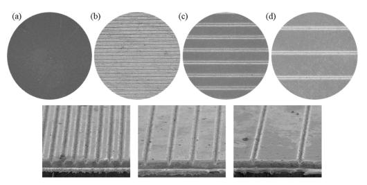
Figure 4. (a) Unstructured, (b) pitch distance of 112  $\mu$ m, (c) pitch distance of 224  $\mu$ m, and (d) pitch distance of 448  $\mu$ m.
