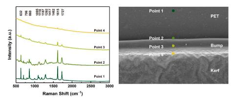
Figure 6. The Raman spectra of PET film after laser processing.
