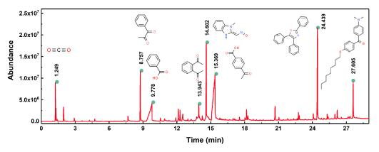
Figure 3. Ion current of evolved gaseous products during pyrolysis of PET film.
