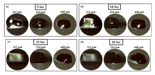
**Figure 7.** Images of the laser structured electrode with pitch distances of 112  $\mu$ m, 224  $\mu$ m, and 448  $\mu$ m, respectively at the time of (**a**) 5 s, (**b**) 10 s, (**c**) 15 s, and (**d**) 20 s.
