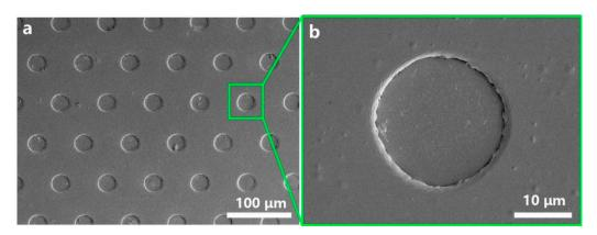
Figure 10. (a) Low- and (b) high-magnification SEM images of the ultra-thin PI film contact spacer.
