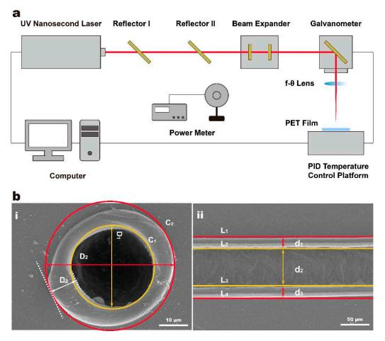
**Figure 1.** The Schematic diagram of the laser processing of PET film (**a**), and the processing quality evaluation (**b**) of different features (hole (i) and kerf(ii)).
