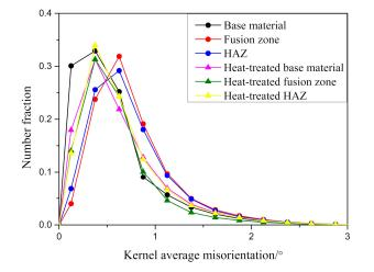
**Figure 10.** Distribution of kernel average misorientation (KAM) of different regions in the as-joined and heat-treated joints.
