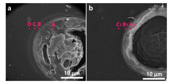
Figure 7. SEM images of the micro-hole (a) before cleaning and (b) after cleaning.
