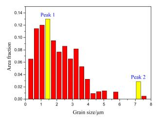
Figure 7. Grain size distribution of the fusion zone in the heat-treated joint (P = 2500 W, t = 5 ms).
