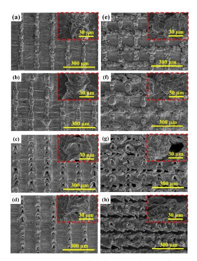
**Figure 3.** SEM micrographs of the laser textured BMG surfaces using different scanning speeds: (**a**–**d**) unidirectional surface patterns with the scanning speeds of 20 mm/s, 40 mm/s, 60 mm/s, and 80 mm/s; (**e**–**h**) cross-hatch surface patterns with the scanning speeds of 20 mm/s, 40 mm/s, 60 mm/s, 60 mm/s, and 80 mm/s.
