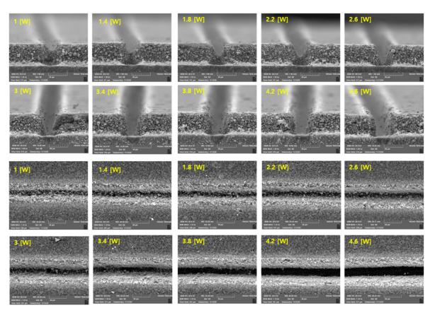
Figure 2. SEM image of the electrode after the laser structuring with two-pass.
