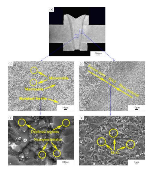
**Figure 4.** Morphologies of the weld seam with filler material: (**a**) SEM morphology of the weld seam, (**b**) fusion zone, (**c**) fusion line, (**d**) enlarged fusion zone and (**e**) enlarged HAZ.
