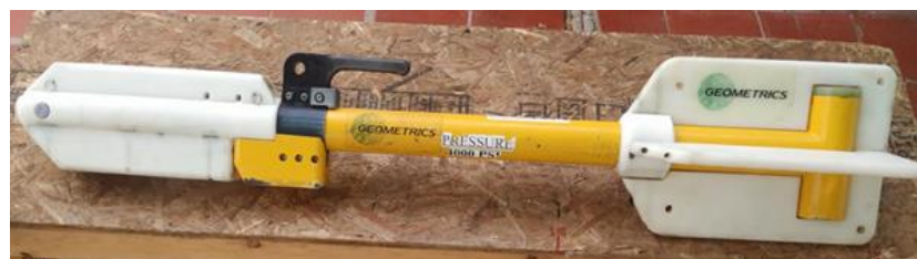
Figure 4. Geometrics G-882 marine magnetometer. Source Karem Oviedo Prada, 2020.
