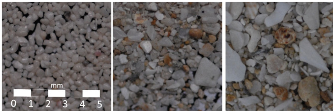
Figure 10. Left panel shows the native sand, 2004. Central and right panels, sand from the emerged and submerged beach fill, respectively.
