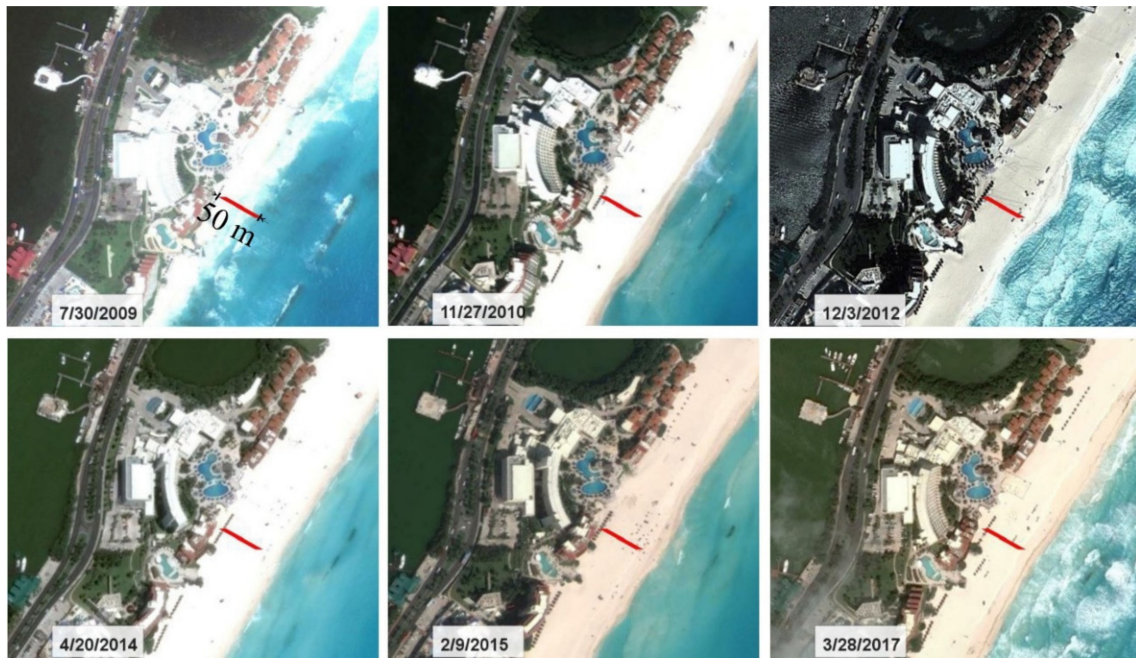
Figure 14. Satellite images, 2009 to 2017, of the beach in front of the Grand Park Royal Cancun, located in the central-north part of the beach (source: Google Earth Pro, version: 7.3.2.5776). The red line, 50 m long, shows the dynamic stability being reached.
