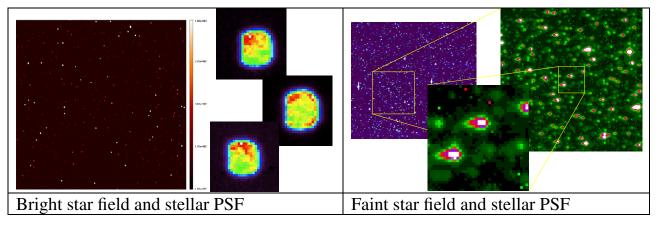
Fig. 1.3.5. Point spead functions in the two CoRoT fields, with the very broad stellar images in the bright star field (to improve the accuracy of the photometry) and the smaller faint star images in the faint star field, enlarged by the very low resolution prism to extract color information, © CNES.
