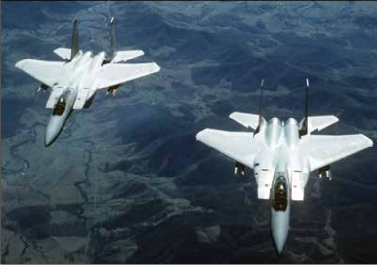
Two Air Force F-15 Eagles. Developed under the Air Force's F-X program, the F-15 was redesigned by Boyd using his energy-maneuverability equation to reduce the aircraft's weight and increase its air-to-air combat performance. Defense Imagery Management Operations Center
