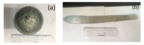
**Figure 6.** The macroscopic appearance: (a)  $(Fe_{0.3}Co_{0.5}Ni_{0.2})_{95}(Al_{1/3}Si_{2/3})_5$  alloy ingot prepared by maglev melting, (b) cold-rolled sheet.
