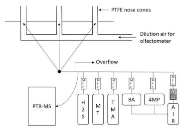
**Figure 1.** Schematic drawing of gas dilution system and connection to the olfactometer. H2S: Hydrogen sulfide; MT: methanethiol; TMA: trimethylamine; BA: butanoic acid; 4MP: 4-methylphenol; PTR-MS: Proton-Transfer-Reaction Mass Spectrometry; MFC: mass flow controller.
