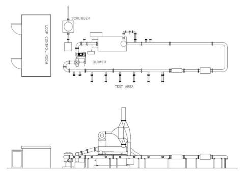
Figure 1. Mechanical dimensions of the LOOP facility.
