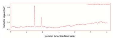
Figure 5. Chromatogram of one of the samples generated with a vaporisation temperature equal to  $270\,^{\circ}$ C; set-up conditions are identical, as in the test showed in Figure 4. In this case, two peaks are present, one at  $1.89\,\mathrm{min}$  and the second at  $1.46\,\mathrm{min}$ .
