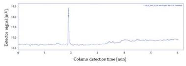
Figure 4. Chromatogram obtained from one of the samples generated with a vaporisation temperature equal to  $140\,^{\circ}$ C; visible pack at  $1.89\,$ min is related to butanol and is verified using a traceable gas standard.
