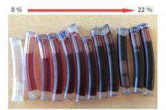
**Figure 9.** Test specimen samples. Tube segments were filled with diluted blood and sealed with hot glue. In order to test the effect of bubbles, a small fraction of air was left inside. This also prevented direct contact between the hot glue and test liquid. Samples were produced for blood concentration between 0% and 22% in increments of 2%. *Hb* concentration was measured using a hemoglobin analyzer.
