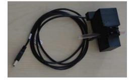
**Figure 8.** Image of the assembled sensor as used in the clinical validation study. Communication and power supply were realized using a USB 3 interface. A short tube segment was inserted to showcase sensor attachment to the CBI system.
