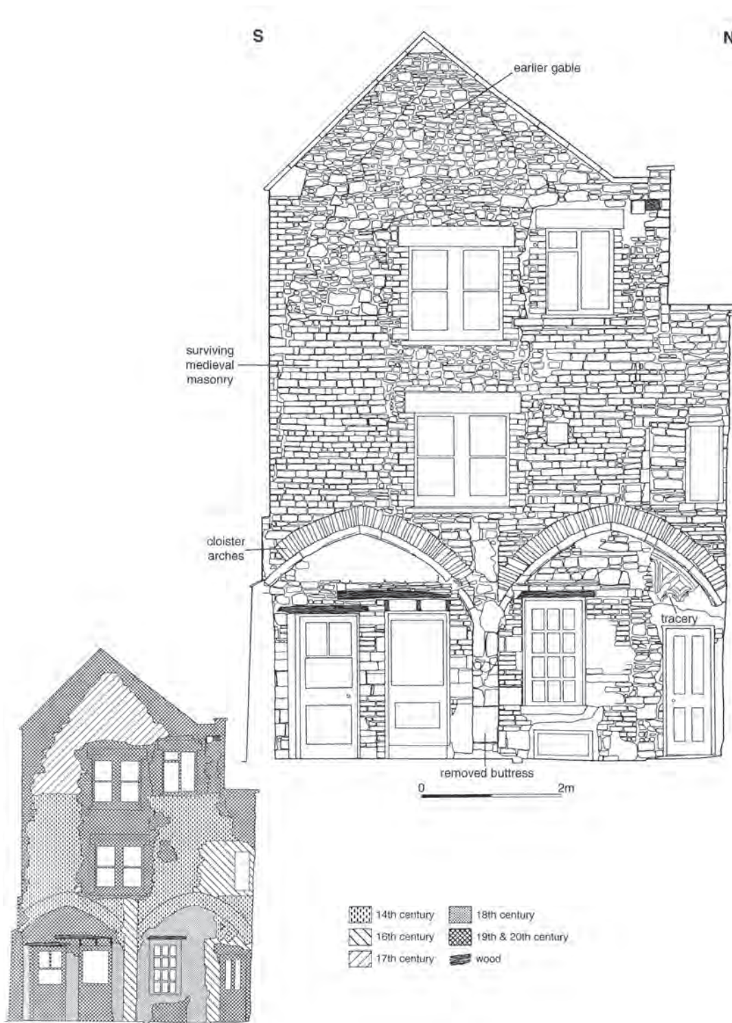
Figure 6.55 Elevation of the rear wall of Church House (reproduced from Jackson 2006b, fig 13, following Bryant 1993, fig 8)
