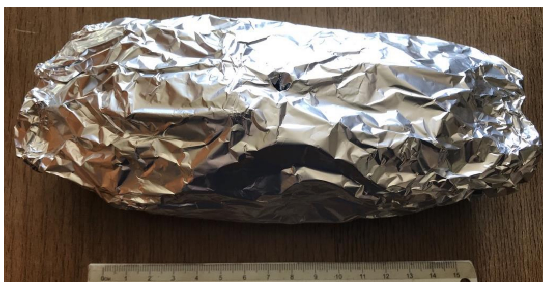
Figure 1. Assemblage of the samples in aluminum foil for torrefaction and pyrolysis tests.
