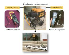
Figure 2. Mechanical and environmental characterization of diesel engine-electrogenerator set [17].
