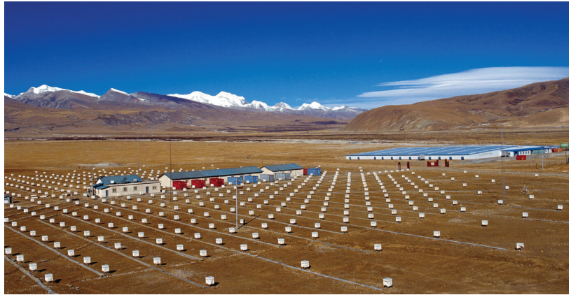
Figure 2. Example of a typical air shower array (Tibet AS \gamma experiment located at the YangBaJing Cosmic Ray Observatory in Tibet (P.R. China) 4300 m asl).
