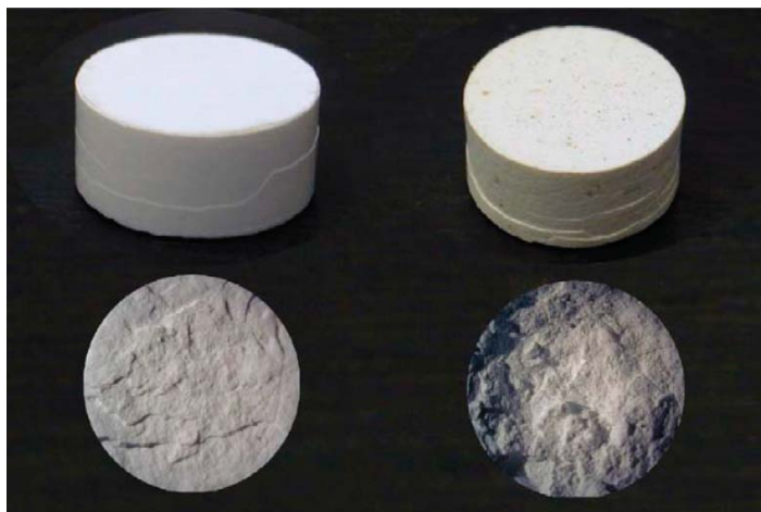
Figure 4. Mg(NH 3 ) 6 Cl 2 for ammonia storage [50].
