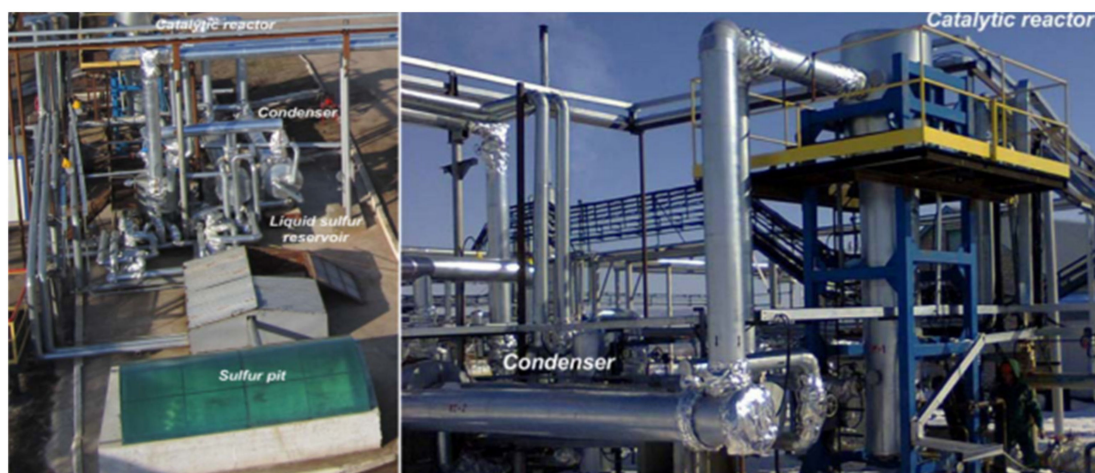
Figure 23. Industrial unit with a capacity of acid gas of up to 250 nm 3 /h, which has been in continuous operation since 2011. The hydrogen sulfide content is 30–65 vol.%.
