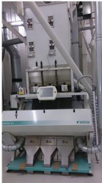
Figure 2. Sortex Z+ Optical Sorter
