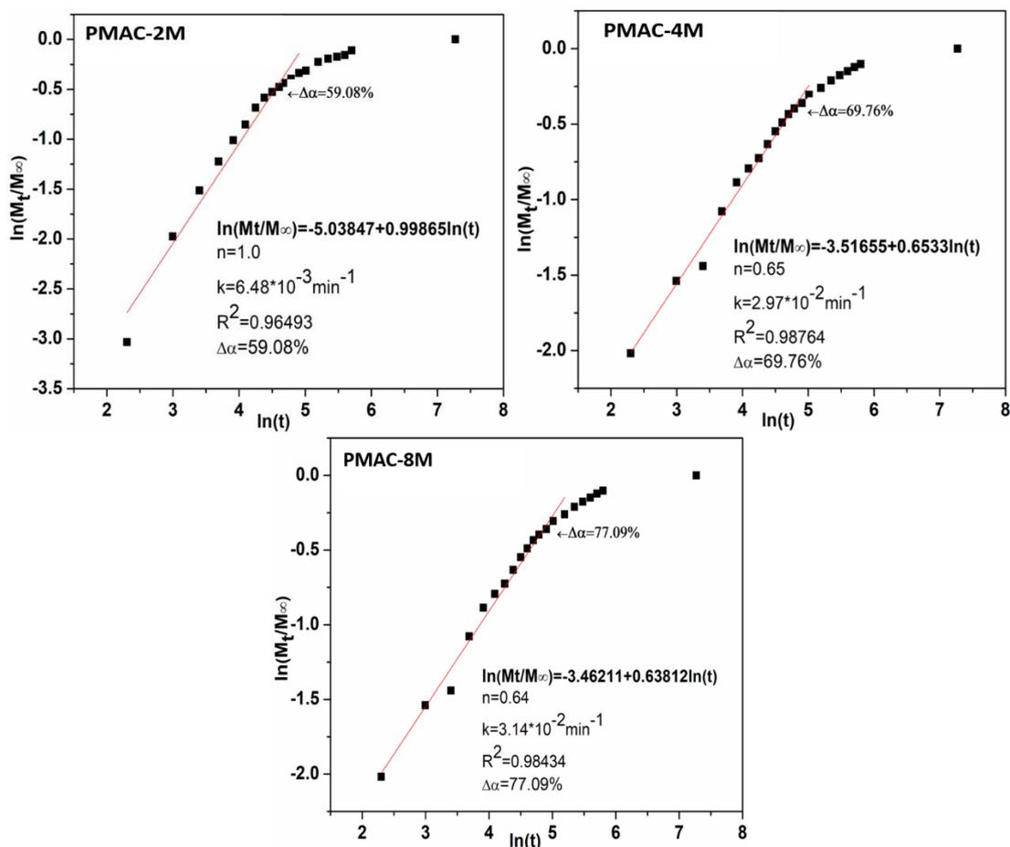
Figure 1. Fitting of the profiles of caffeine release from the PMAC carriers in PB 6.8 with R-P model
