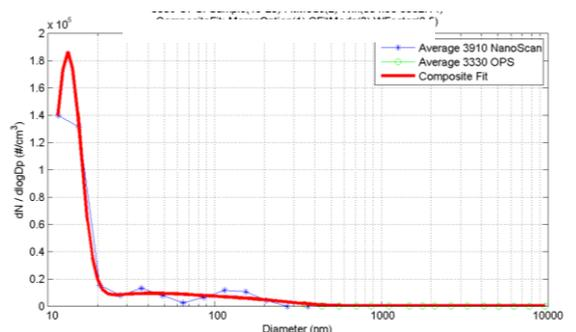
**Figure 1:** Example of a number-size distribution of a vacuum cleaner using a paper bag.
