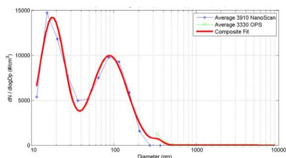
**Figure 2:** Example of a number-size distribution of a vacuum cleaner using a water tank.
