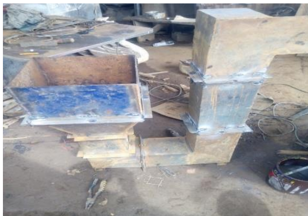
Figure 8: Fabrication of the Iron Ore Sintering System.
