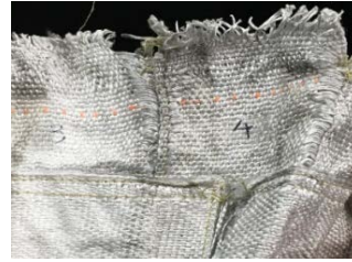
Fig. 3. Protective sheet after rupture
