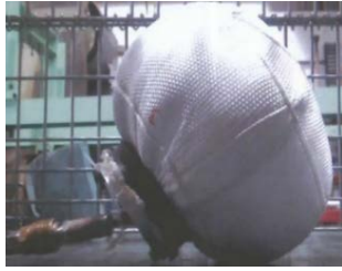
Fig. 2. Two-layered pipe plug used in the ruptured test
