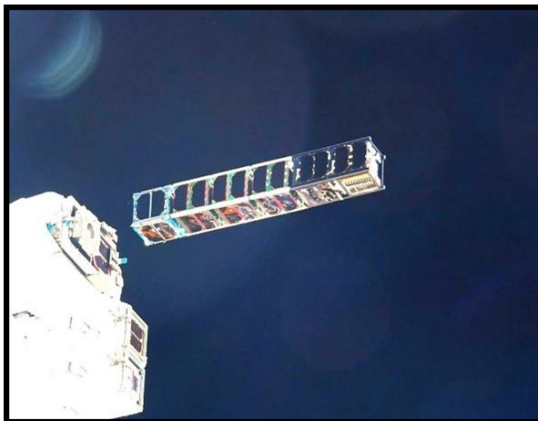
Figure 49 Birds-4 satellites deployment from the International Space Station. This Deployment Image was taken by Astronaut Soichi Noguchi from ISS [51]
