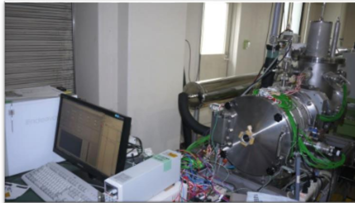
Figure 40 Vacuum chamber used in the experiment with aged perovskite solar cells
