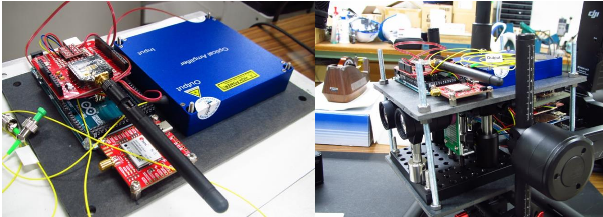
Figure 6-13: EDFA mounted close to the GPS module
