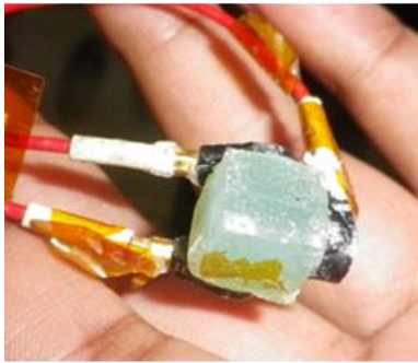
Figure 5-10: Piezo Accelerometer sensor placement and axes
