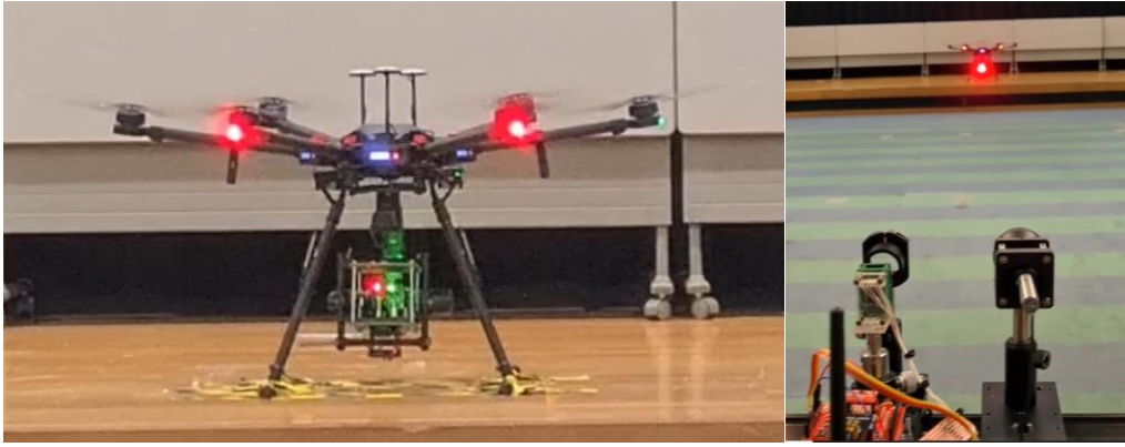
Figure 6-15: Laser beam from the Drone lasercom module illuminating the receiver.
