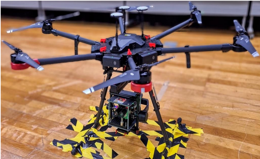
Figure 6-1: Hexacopter Drone with Fitted Lasercom Module
