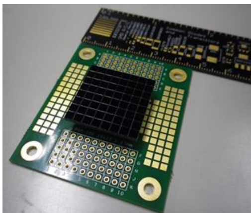
Figure 4-8: Photodiode Array assembled on a BGA adapter
