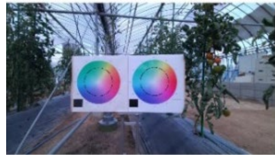
Fig. 6 The experimental setup to measure the effects of sunlight. The polarizing films are attached to the one of camera and the light to be perpendicular to each other.
