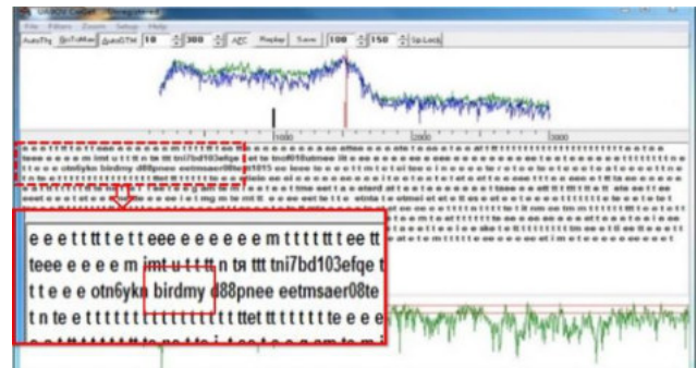
Figure 6. UiTMSAT-1's beacon reception display on CWGet. The dotted box was zoomed-in to display the text "BIRDMY". BIRDMY was the UiTMSAT-1's satellite identification
