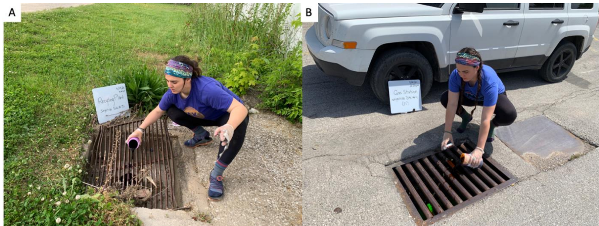
Figure 17: Injecting Dye into storm drains in Horse Cave, KY.
