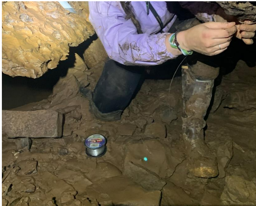
Figure 16: Attaching a receptor to a rock using monofilament line.
