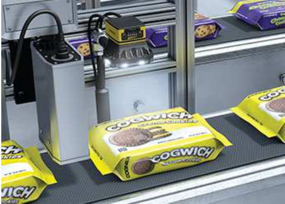
Figure 25. Lighting in vision systems (Cognex, 2021).
