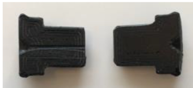
Fig. 8. Filed groove in one piece of capillary holder module.
