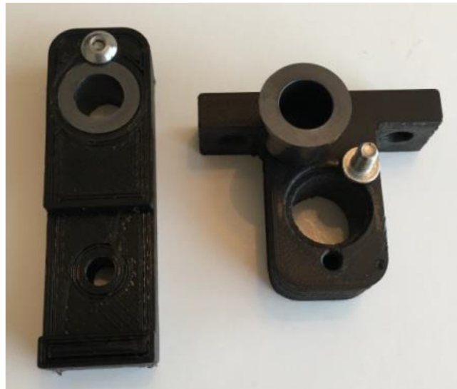
Fig. 9. Press-fit and secured bushing into X, Y-axis lead screw supports.
