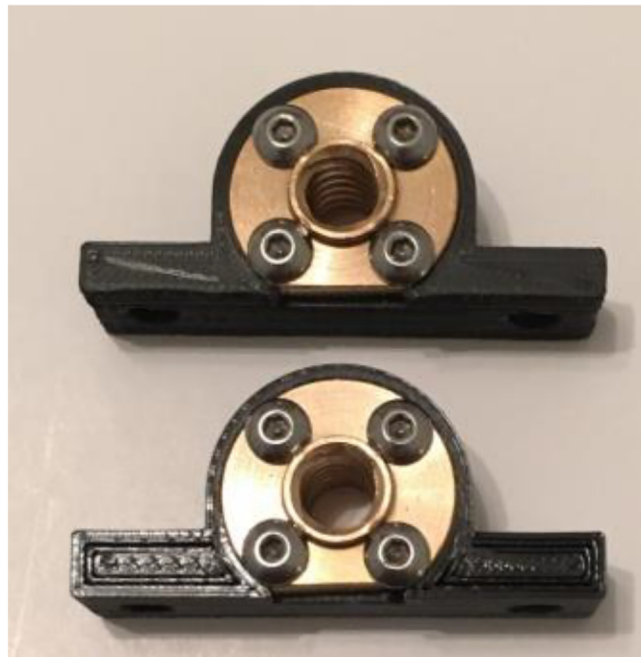
Fig. 10. Secured X,Y-axis lead screw nuts in housings.
