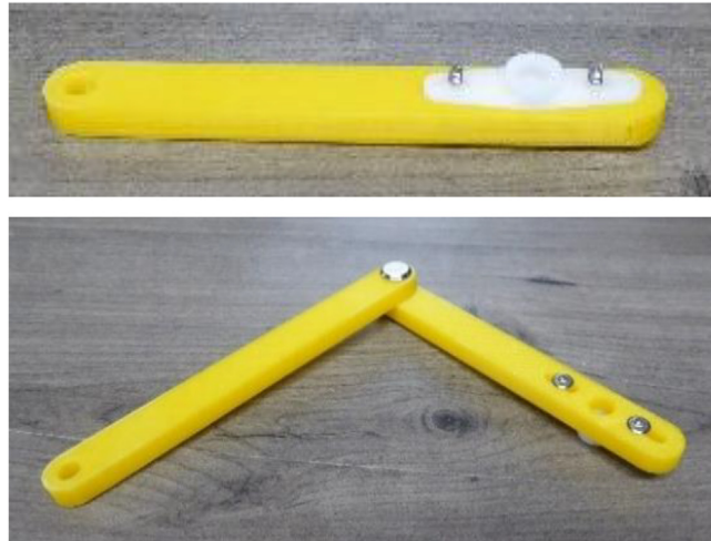
Fig. 44. Link B1 connected to the R-I horn (top) and connection between links B1 and B2 (bottom).
