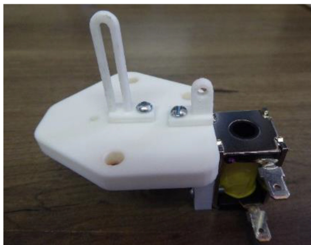
Fig. 41. Capillary rail and lever pivot attached to top of capillary plate.
