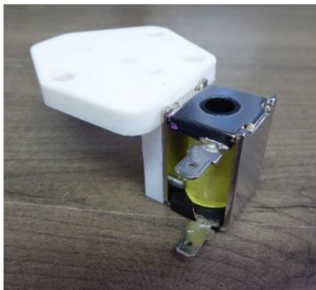
Fig. 40. Connection of end effector to solenoid coil body.
