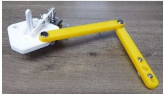
Fig. 45. Connection of capillary plate and right sub-linkage.
