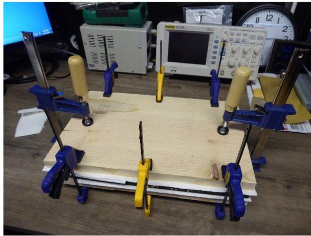
Fig. 31. Tightened clamps used to hold the base stack together for glue curing.
