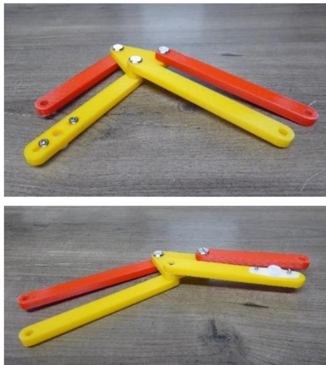
Fig. 47. Top view (top) and underneath view (bottom) of the elbow connected to links A1, A2, P1, and P2 (complete left sub-linkage).
