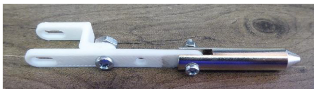
Fig. 42. Combined lever and plunger assembly.
