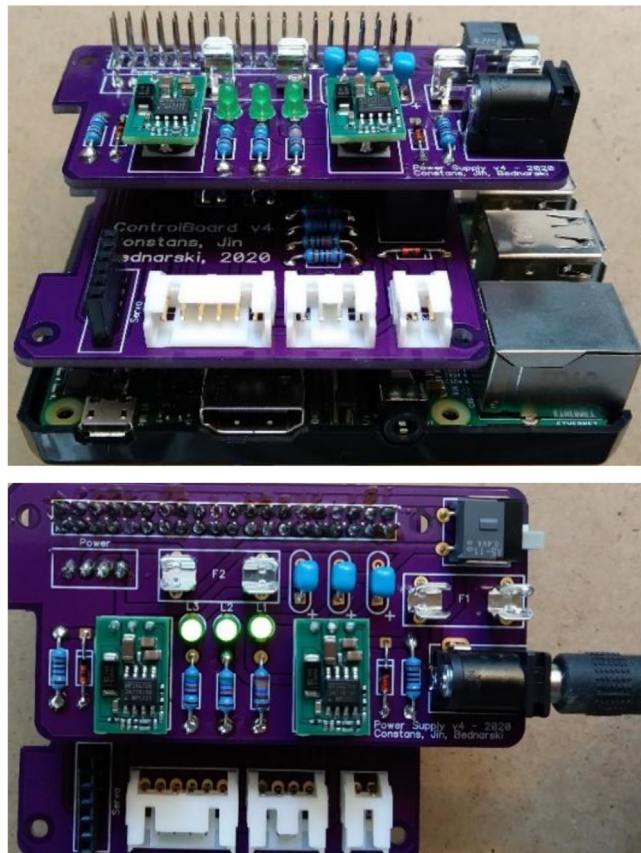
Fig. 52. Stack of Raspberry Pi, control board, and power supply board (top). Three LEDs light up when power supply board is plugged in and power switch is turned on (bottom).
