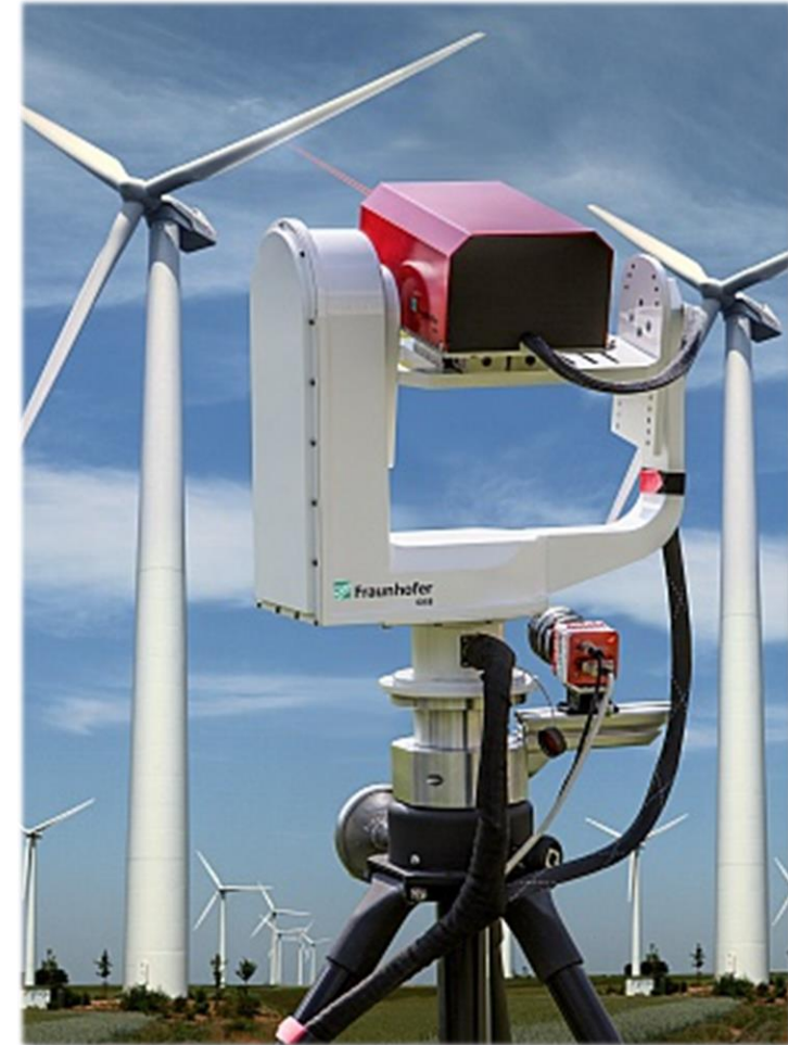
Wind turbine monitoring using LDV as a non-contact approach (Fraunhofer Institute of Optronics).
