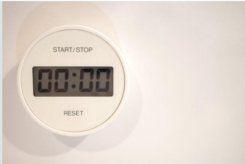
Figure 5: Kitchen timer released by Muji, designed by Hiroshi Seki and Yohei Kuwano. The functionality offered is minimal: Start/Stop and Reset are buttons, and time is adjusted by rotating the outer dial. Photograph by the author.
