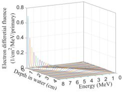
Figure 7: Electron differential fluence at different positions through the water sample container.
