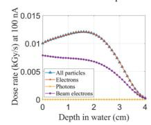
Figure 6: Dose contributions resulting from the electrons and bremsstrahlung photons.
