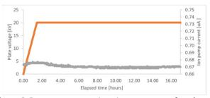
Figure 5: Ion pump current (gray) response as a function of time when voltage (orange) is applied to both electrode plates simultaneously.
