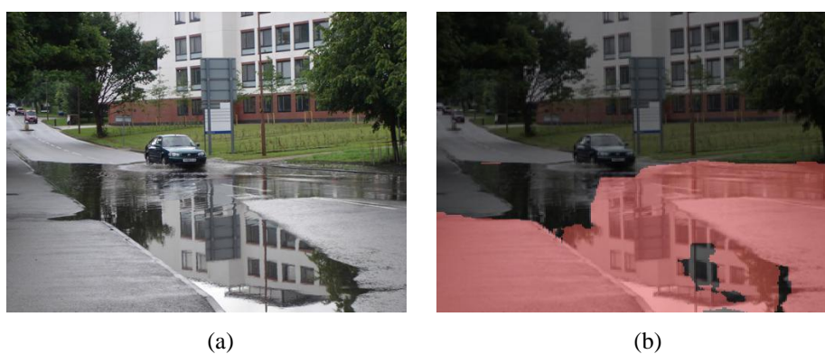
Fig. 12. (a) Original and (b) segmented image of a suburban scene. Segmented flood regions are overlaid red
