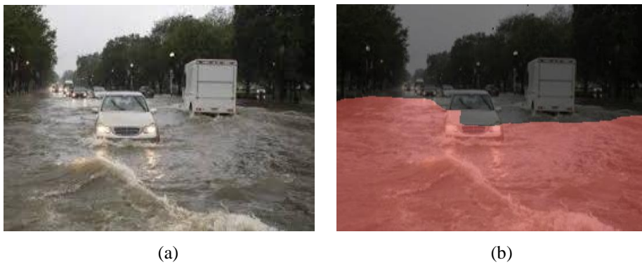
Fig. 14. (a) Original and (b) segmented image of a roadway with a red overlay.
