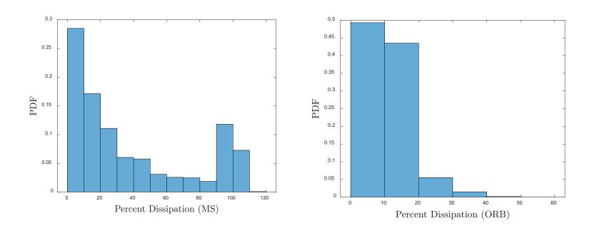
Marsh sill shows a variety of wave dissipation rates while oyster reef ball shows mostly small dissipation rates.
