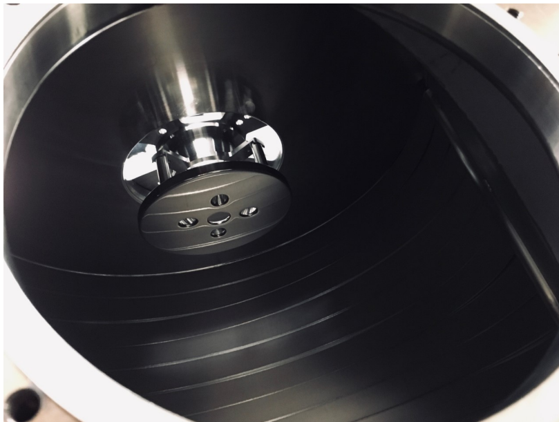
FIG. 115: Anode assembly and thin NEG stripes at the bottom of the gun chamber.
