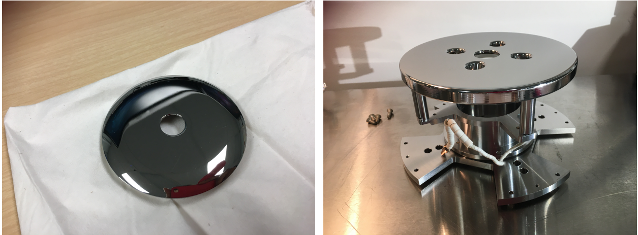
FIG. 114: Flat cathode front (left) and flat anode plate mounted on to the outer flange (right).
