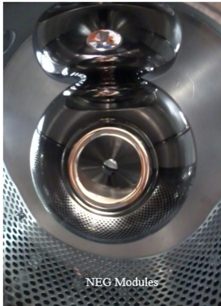
FIG. 13: The NEG modules inside the gun chamber.
