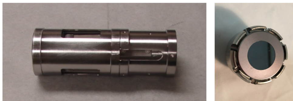
FIG. 8: Photograph of the locking device used to hold the photocathode puck (left) and the puck with tantalum cup holding Mo substrate (right).
