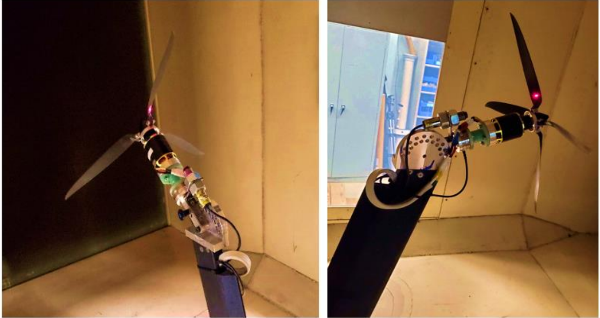
Figure 20. 3 and 4-blade propeller configurations in low-speed section.
