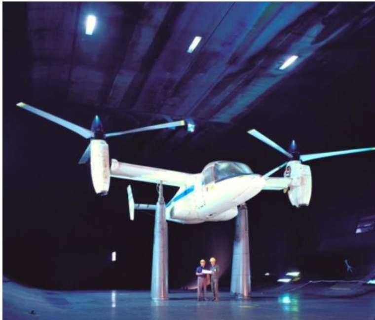
Figure 10. The XV-15 in the NASA Ames 40×80-ft. wind tunnel [5].
