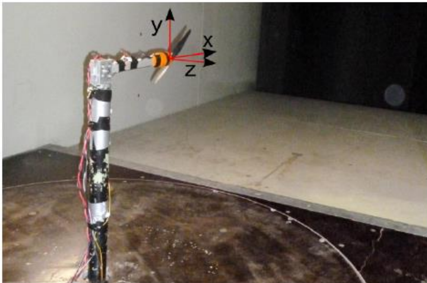
Figure 11. Theys test rig mounted on turntable inside wind tunnel [20].
