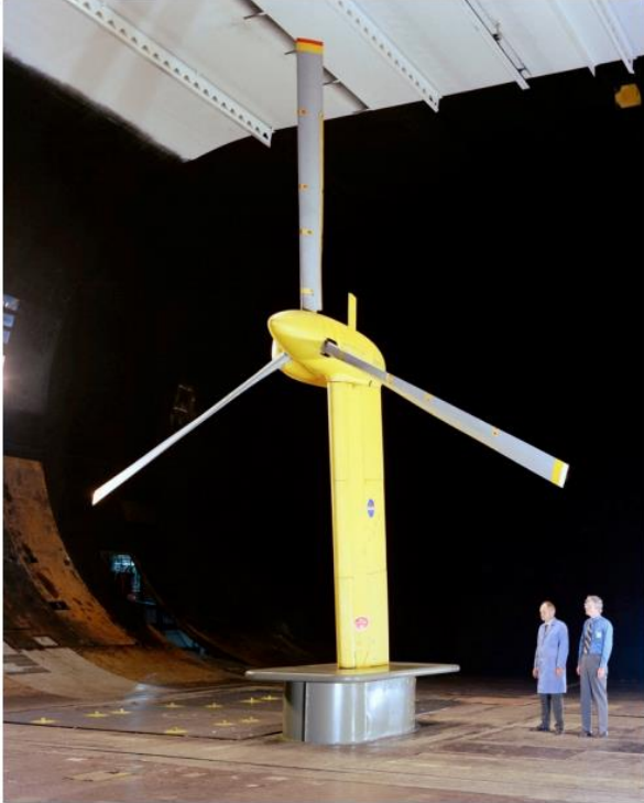
Figure 9. Bell 25-ft. diameter propotor on semi-span wing in NASA Ames 40×80-ft. wind tunnel [5].
