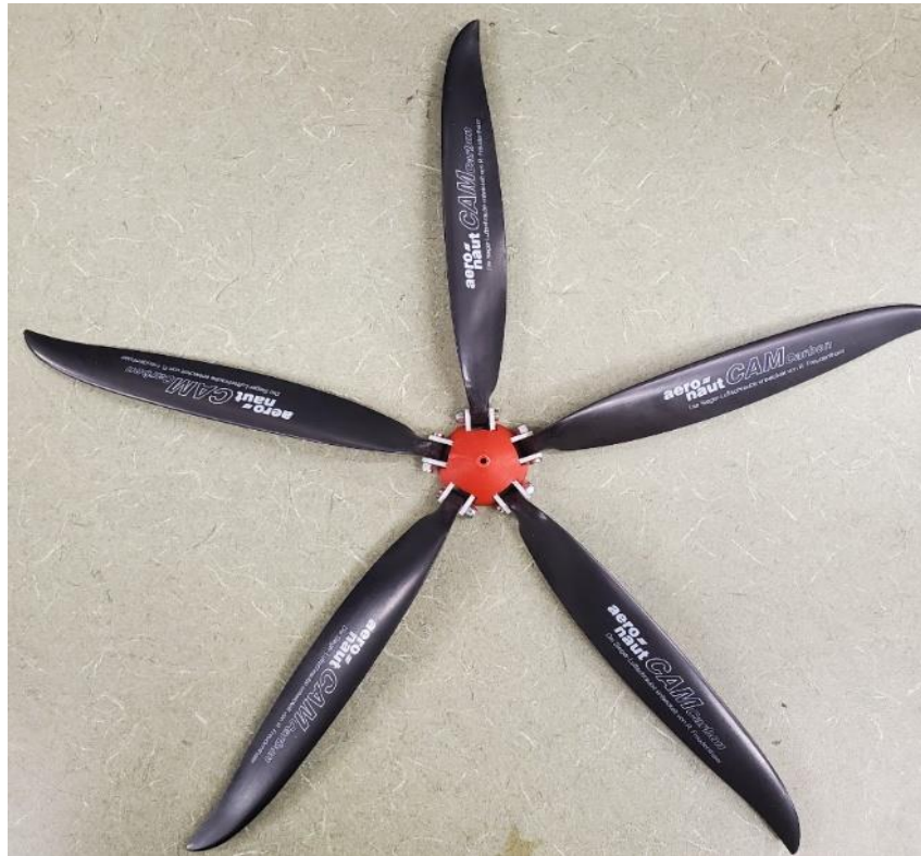
Figure 22. Aeronaut CAM Carbon blades in 5-blade propeller configuration.
