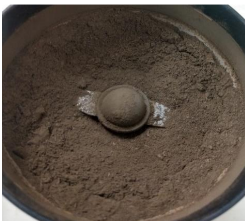
Figure 6. UHS generated through enzymatic hydrolysis of pretreated corn stover
