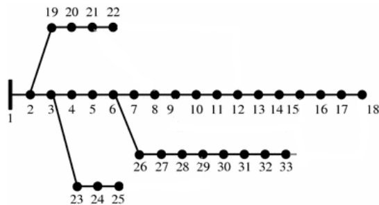
Fig. 3.9: IEEE 33-bus distribution test system.
