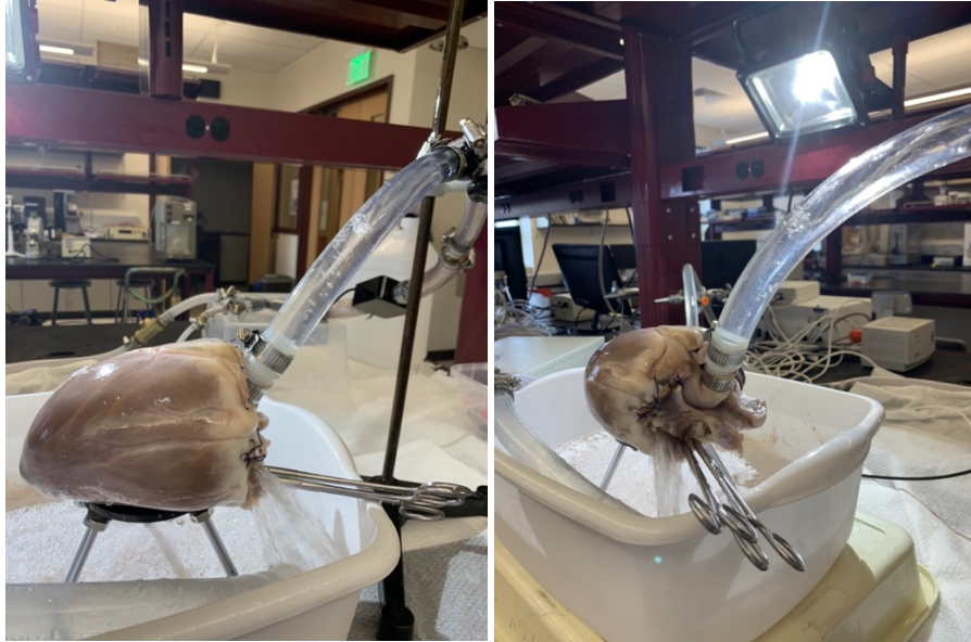
Figure 3.1.5: Heart connected to Steady Flow System. Left atrium is unattached from tubing of the system and propped up, ensuring that the LV and LA are continuously filled with fluid, with no air trapped inside.
