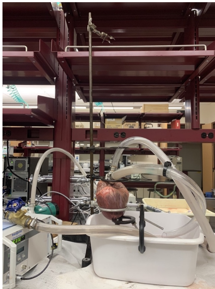
Figure 3.1.4: Ex vivo Steady Flow System.
