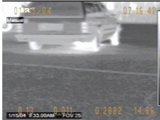
Figure 19. Blue with 0.13 %CO. The vehicle would still pass an emissions test, but is still warming up.
