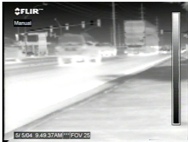
Figure 35. Hot SUV. The reflection can be seen on the road, but the right edge of the reflection blends in with the road reflection.
