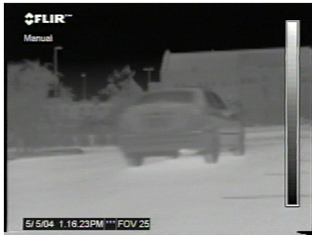
Figure 41. The vehicle is noticeably warmer than the previous figure. The reflection, the exhaust system, and the tire treads are brighter. This image was taken 39 seconds after Figure 40.
