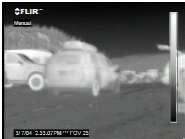
Figure 31. Cold SUV leaving the parking lot. The SUV in this figure looks very similar to the Breckinridge Ski Patrol vehicle; however the hot looking tire wall is due to heating by the sun and not by being driven. This can be determined because the other tire walls do not look hot.
