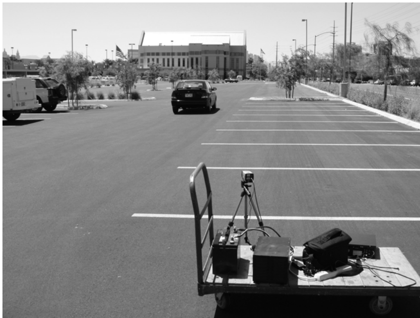
Figure 9. Set-up in DRI parking lot for observing the cold start vehicle warming up as it was driven around the parking lot.
