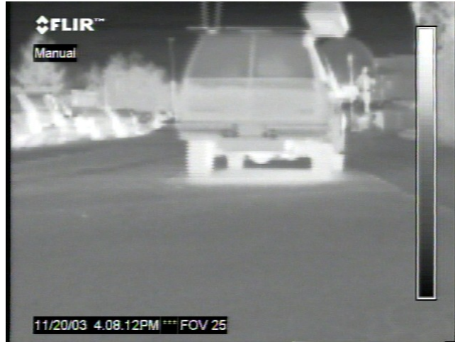
Figure 26. Hot Sport Utility Vehicle. This vehicle has both hot tire treads as well as a very bright reflection from the underbody of the vehicle.
