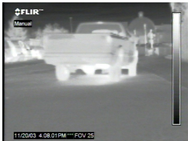
Figure 25. Hot truck. Has a very bright reflection under the vehicle as well as uniformly heated tire treads and sidewalls on the tires.
