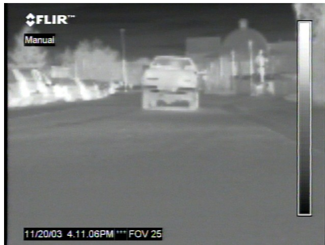
Figure 27. Hot truck. The truck in this image has both hot tire treads and a bright reflection from the underbody of the vehicle. The reflection can be seen at a distance as long as the road surface is level.
