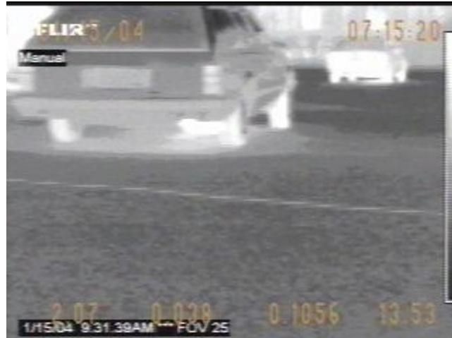
Figure 17. Blue, with %CO of 2.07. The reflection from the underbody of the vehicle is much stronger than the previous figure.
