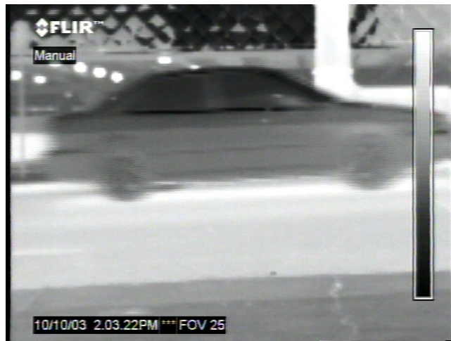
Figure 13. Hot vehicle driving east on Iliff Avenue. There is a bright reflection from the underbody of the vehicle, but the tire treads cannot be seen to further determine the status of the vehicle.
