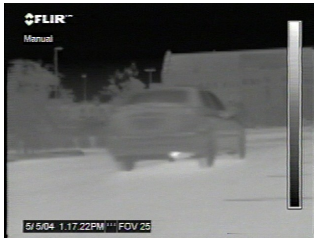
Figure 43. The tailpipe of the vehicle is very noticeable; however the reflection does not appear to be getting any brighter.
