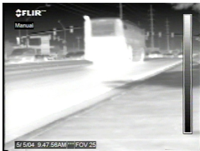
Figure 34. Citizens Area Transit (CAT) Bus. The engine location for the bus is in the rear of the vehicle. The bus is obviously hot, and the exhaust pipe location can be seen through the body of the bus.
