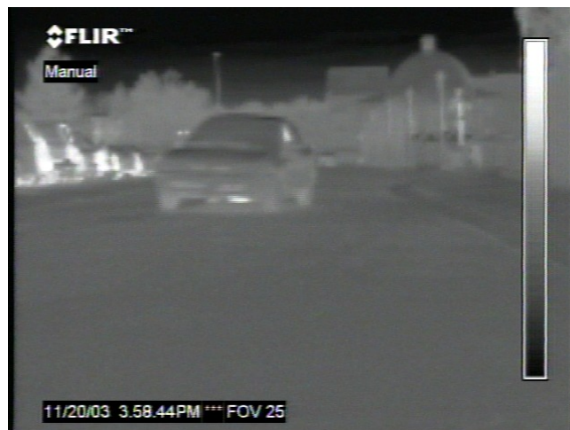
Figure 21. Cold vehicle. This vehicle is leaving the restricted parking lot across from the north side of Olin Hall, and has no bright underbody reflection or hot tire treads.
