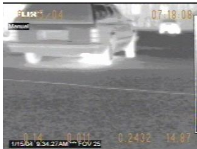
Figure 20. The vehicle is still emitting a constant percentage of CO in the exhaust, and is now fully warmed up.
