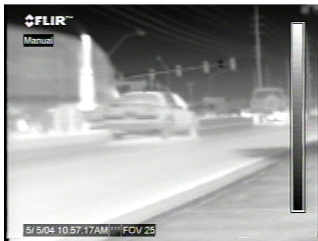
Figure 36. Cold DRI employee vehicle. This vehicle is known to have been sitting long enough to reach the ambient temperature, however the high temperature and the driving time, approximately 20 seconds, from the parking lot to the road was enough for the vehicle to warm up noticeably.
