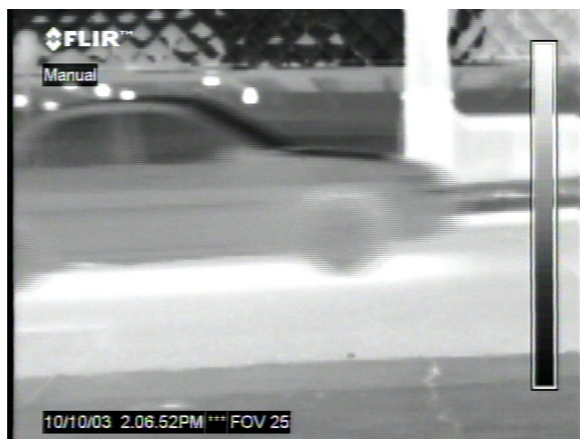
Figure 14. Hot vehicle. This vehicle has both a bright reflection from the underbody of the vehicle as well as warm side walls on the tires.
