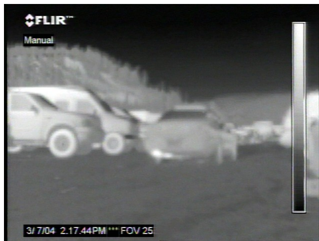
Figure 29. Warm vehicle leaving the parking lot. The exhaust system of this vehicle appears to be hot, however because there is no reflection on the road surface on the snow, the status of this vehicle cannot be clearly determined.
