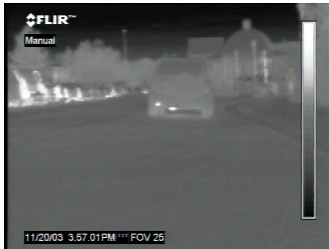
Figure 22. Cold start vehicle. This SUV has a very faint reflection from the underbody of the vehicle and the tire treads do not emit very much infrared radiation.
