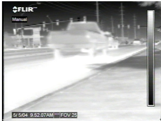
Figure 38. Hot truck. The truck in this image is hot. However the reflection from the underbody of the vehicle is masked by the emission from the road.
