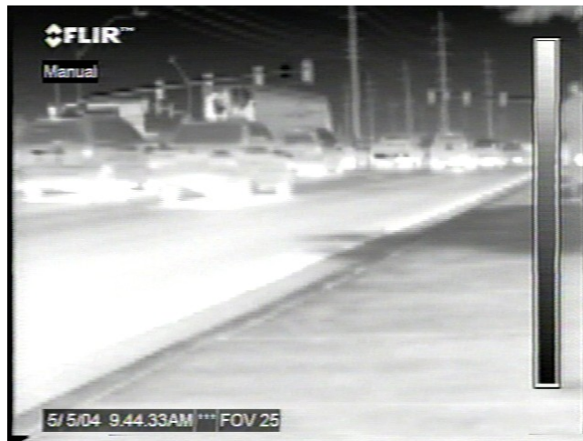
Figure 33. Traffic on Flamingo Road. The vehicles traveling east on are all hot and the reflections from the underbodies of the vehicles can be seen in the lanes.
