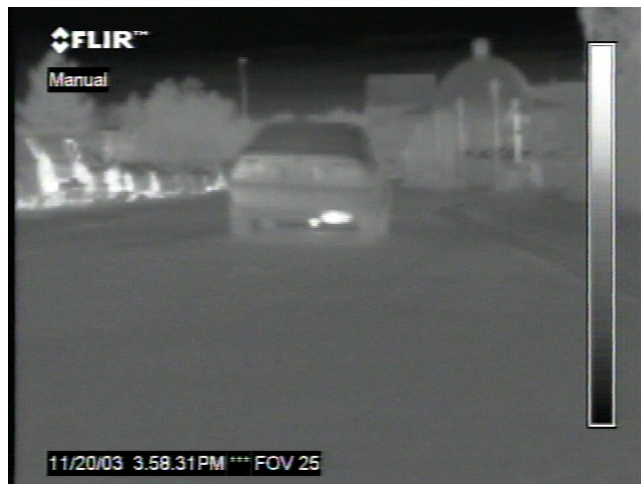
Figure 23. Cold start vehicle. This vehicle is leaving the metered visitor parking lot (304) across from Cherrington Hall, and the exhaust of the vehicle appears to be hot due to the small increase of heat from the vehicle starting. This vehicle has no strong reflection from the underbody of the vehicle or hot tire treads to indicate that it is warm.
