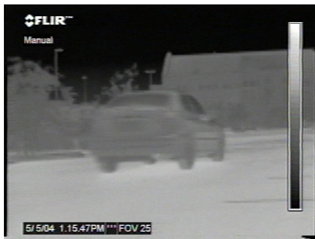
Figure 40. Vehicle after driving around the parking lot one time. The tires and the exhaust system have warmed up and the reflection from under the vehicle can be seen on the road surface. Approximately 49 seconds after start.
