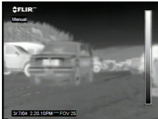
Figure 28. Breckenridge Ski Patrol SUV. The vehicle is hot, as can be seen by the hot engine through the grille, however because snow does not reflect IR radiation, there is no reflection on the road from the underbody of the vehicle.
