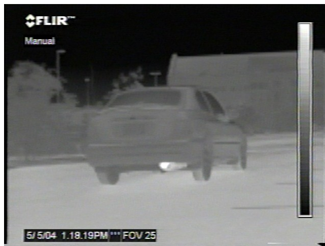
Figure 44. The tailpipe is the brightest object in the image, and the vehicle is fully warmed up. The reflection seems to have reached its brightest more than a minute previous to this image, but the tailpipe continued to get hotter.
