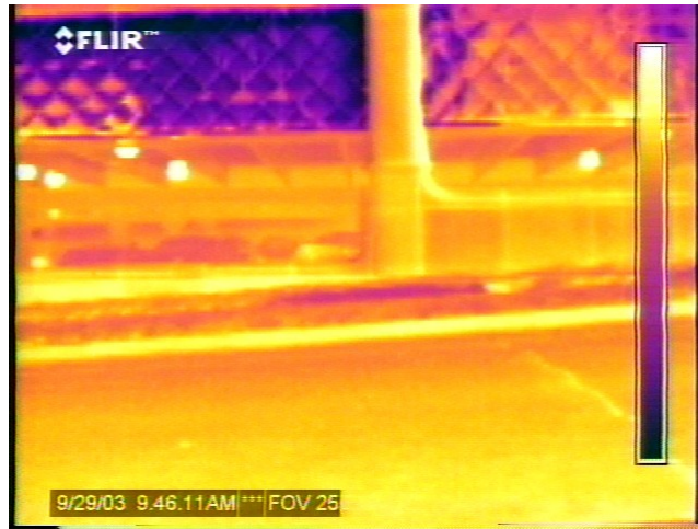
(E) The camera is no longer adjusting the scale of the image.
