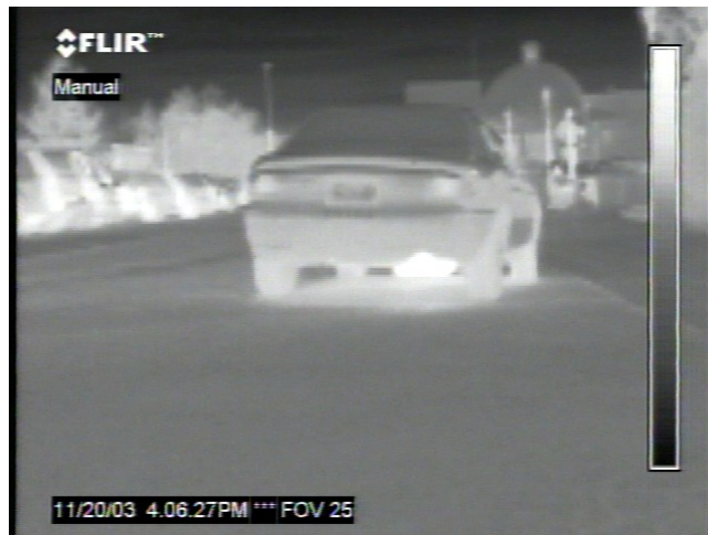
Figure 24. Warm vehicle. It is unknown if the vehicle is fully warm. If the emissions for this vehicle were known, then the status of the vehicle could then be decided.
