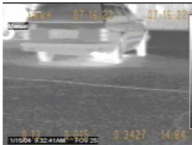
Figure 18. Blue with 0.13 %CO. The vehicle has a much stronger reflection from the underbody of the vehicle, as well as a very bright exhaust system. The vehicle's emissions are now low enough to pass an emissions test. Blue took 224 seconds to warm up.
