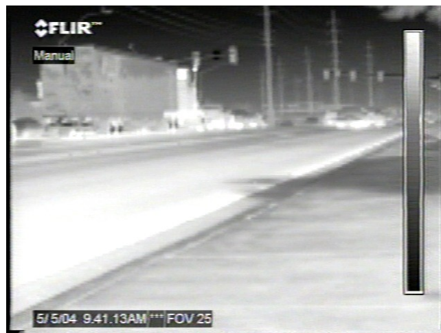
Figure 32. Flamingo Road in Las Vegas, Nevada facing towards the east. The road temperature is over 120°F.
