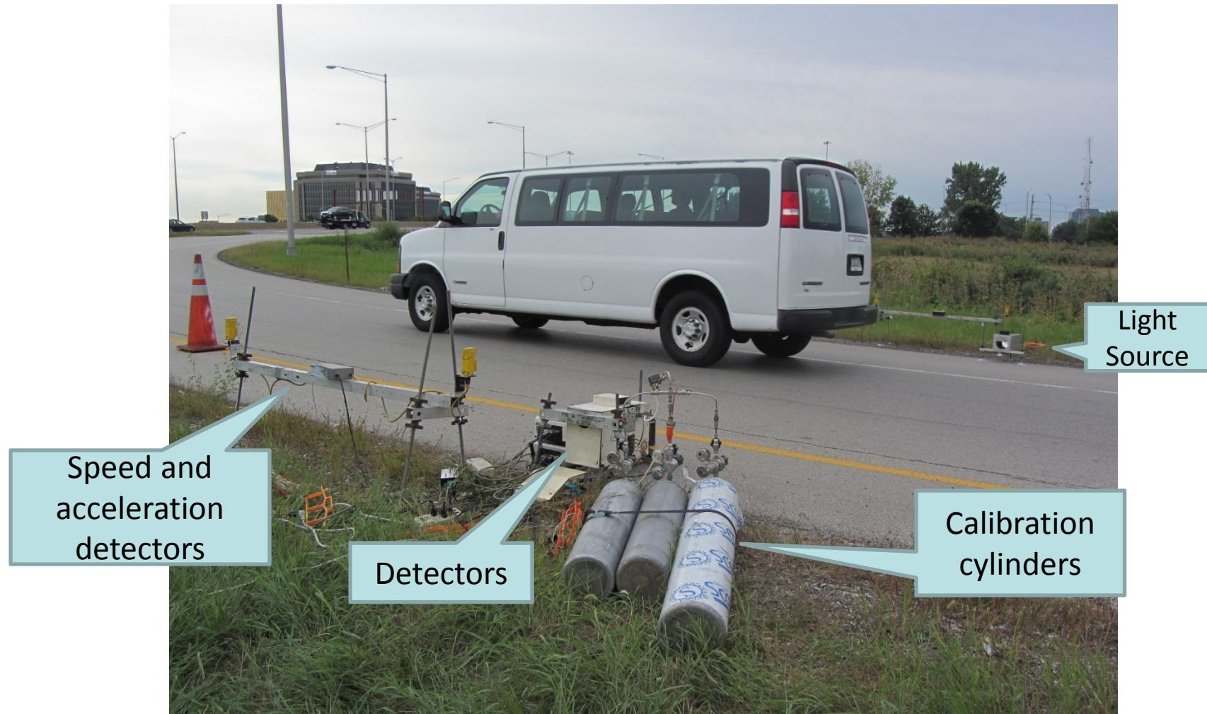
FEAT measures fuel specific (g/kg of fuel) emissions for CO ( $\pm 4$  g/kg), HC ( $\pm 4$  g/kg), NO ( $\pm 0.4$  g/kg), NH<sub>3</sub> ( $\pm 0.05$  g/kg) SO<sub>2</sub> and NO<sub>2</sub> ( $\pm 0.2$  g/kg).
