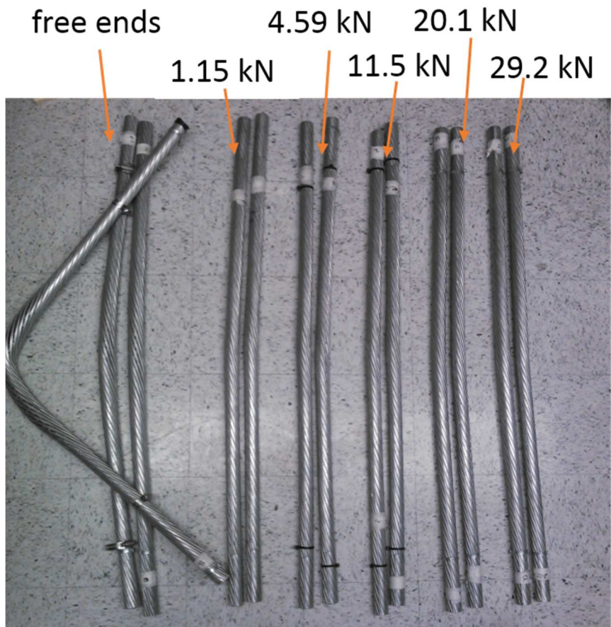
Figure 2-12: Resulting deformation of tested conductors.
