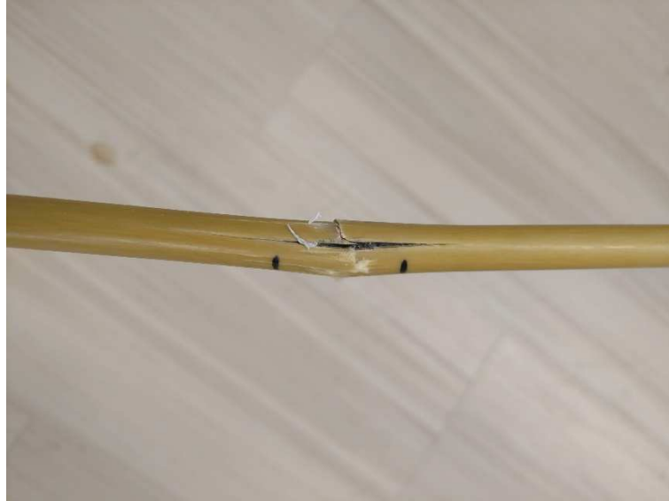
Figure 3-7: Typical example of experimental failure proximal to loading pin in three-point and four-point bend experiments.
