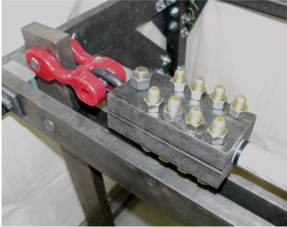
Figure 2-2: Conductor clamp and cable tensioning.
