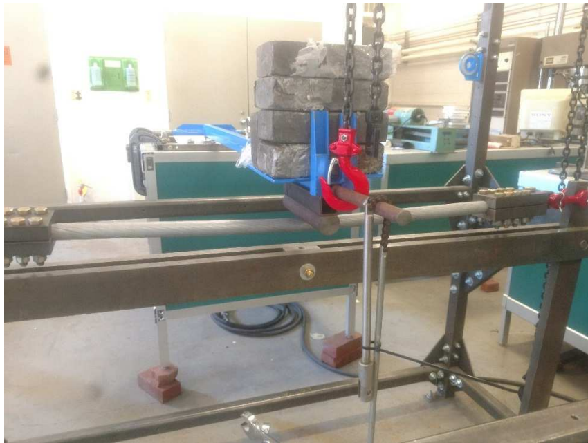
Figure 4-4: Tensioned three point bend setup for ACCC® rod and conductor.
