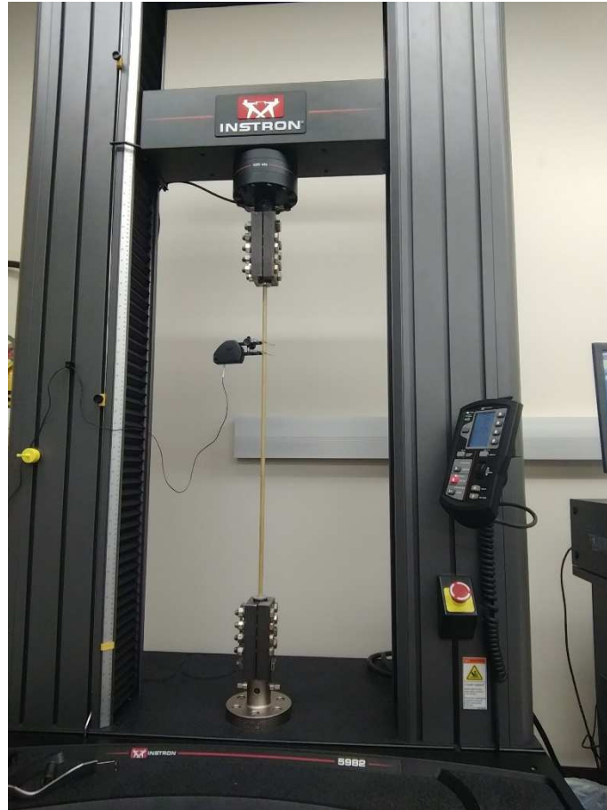
Figure 4-3: Tensile testing of ACCC® rod with FBG array mounted to surface.
