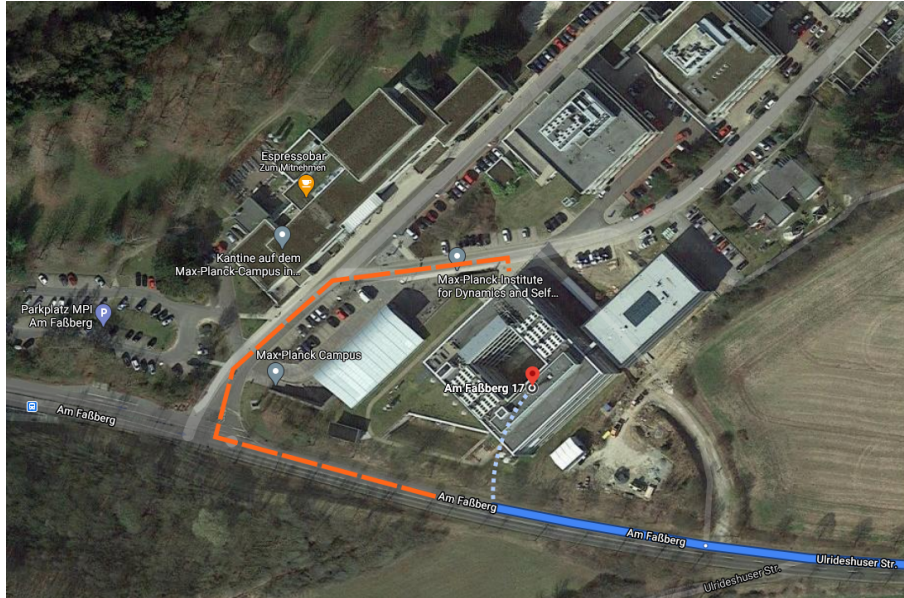
Figure 2.3.: Road snapping based on perpendicular distance from Google Maps shows an insufficient snapping point without direct access to the building. The orange dashed line shows the correct access to the building. The dotted line depicts the access to the building by Google Maps [27].
