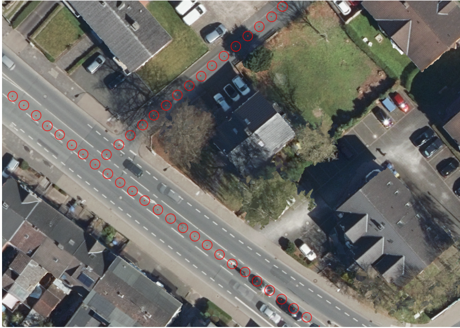
Figure 6.2.: Extract from AOI with the generated source cells as the centroid of the red circles. These source cells were generated with a spacing of 3 meters. This resolution is considered sufficient for accurate snapping.
