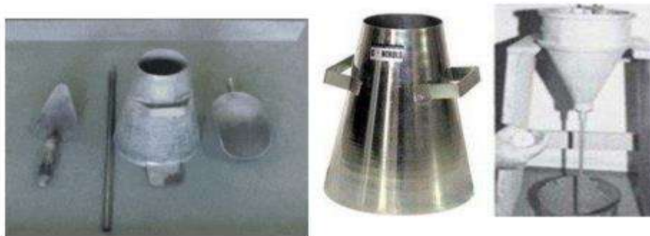
Fig1: equipment for flow slump experience (Prof. Dr. Nabeel Al-Bayati, 2017)
