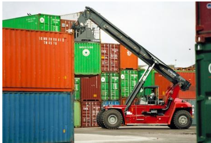
Figure 4.15. Reach stacker operation.
