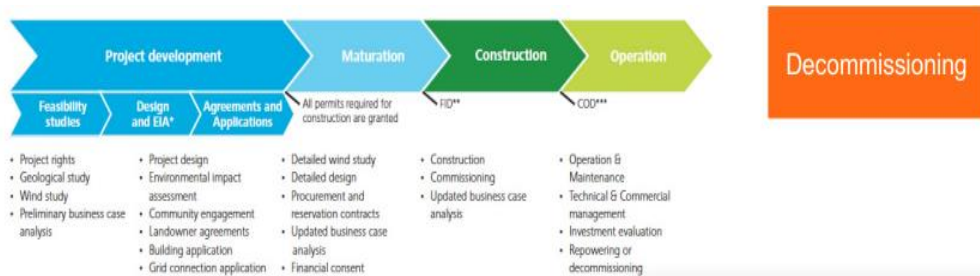
Figure 37: Various phases of a wave farm
